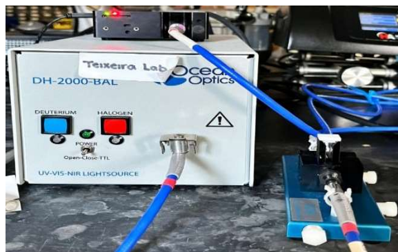
Figure 8. Light source and cuvette utilized to obtain UV-vis intensity data for calibration curve and trials.
