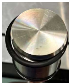
Figure 21. Deformed O-ring on metal syringe after letting acetone sit for an hour.
