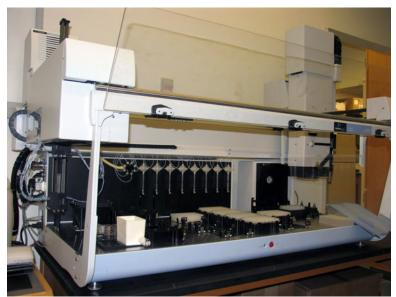
**Figure 3: Photo of the JANUS<sup>TM</sup> Automated Liquid Handling System.** This robot completely automates liquid pipeting tasks allowing analysts to move on to more pressing tasks. (Source: <u>http://www.roswellpark.org/Research/Shared\_Resources/small-molecule-screening-core/smsc-infrastructure</u>)
