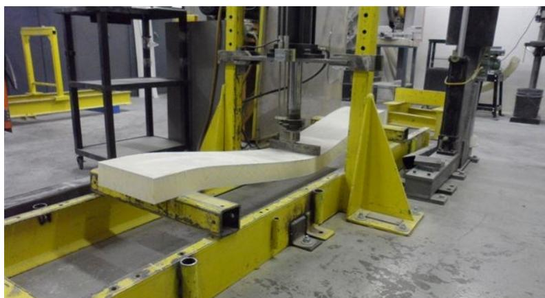
Figure 1-1 Creative Pultrusions Bending Test configuration with failed sample
