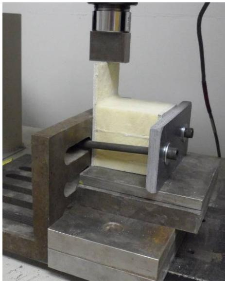
Figure 1-7 Creative Pultrusions Edge Loading configuration
