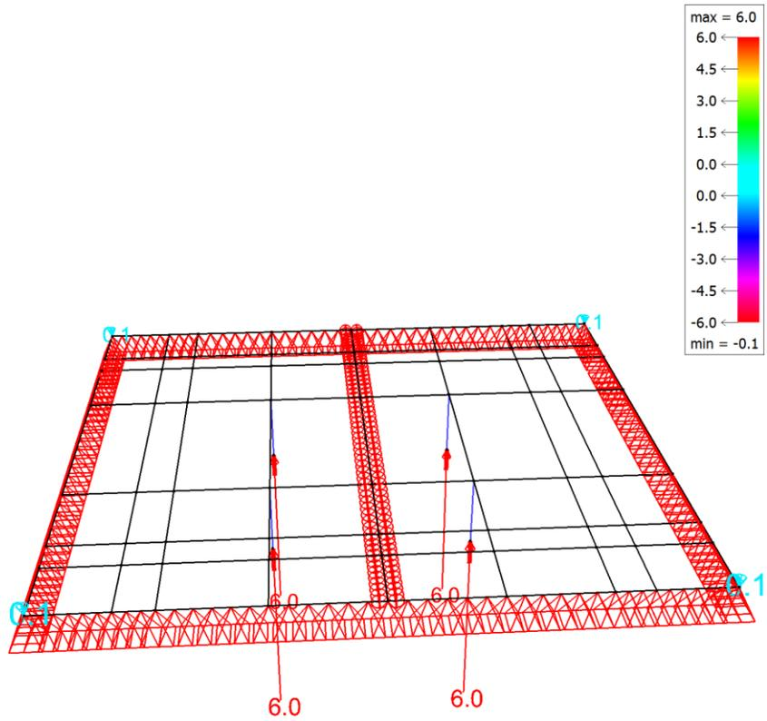
Figure 14: Reaction forces given by the FEA model on the struts (LC 2a) (forces in kN) (BuildSoft)
