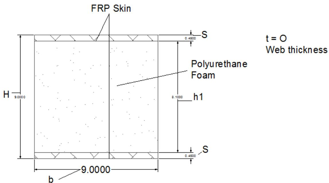
Figure 6 Cross section of Transonite™ Panel in centimeters
