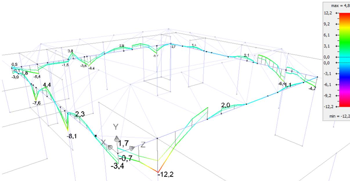
Figure 23: Compression stresses in FRP bottom chord (stresses in N/mm<sup>2</sup>) (Thomas Tassignon) (BuildSoft)
