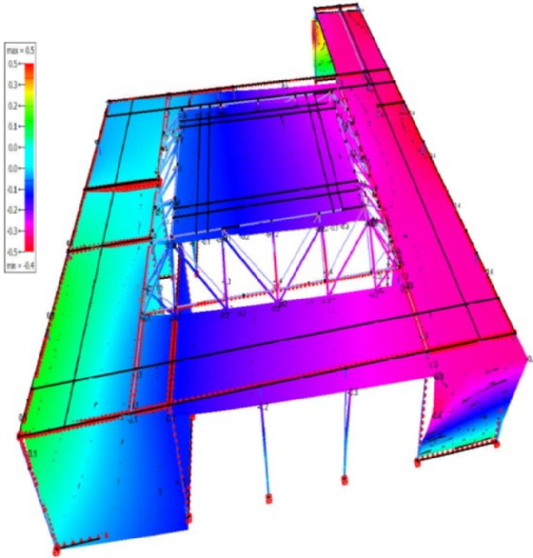
Figure 46 Seismic Deflection in mm (loading applied south to north) (BuildSoft)
