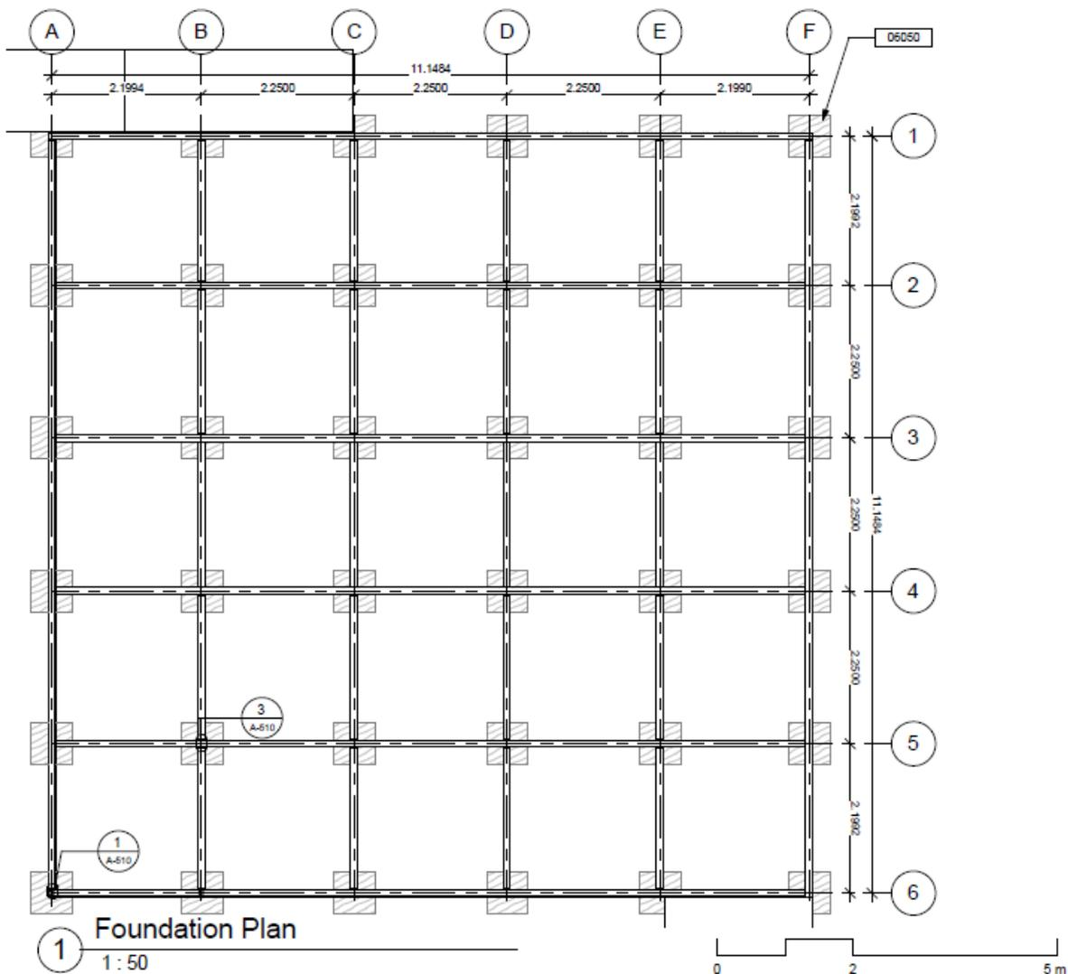
Figure 34 Foundation grid plan (BIM Report submitted to SD China 2013 by Team BEMANY on 3/6/2013)
