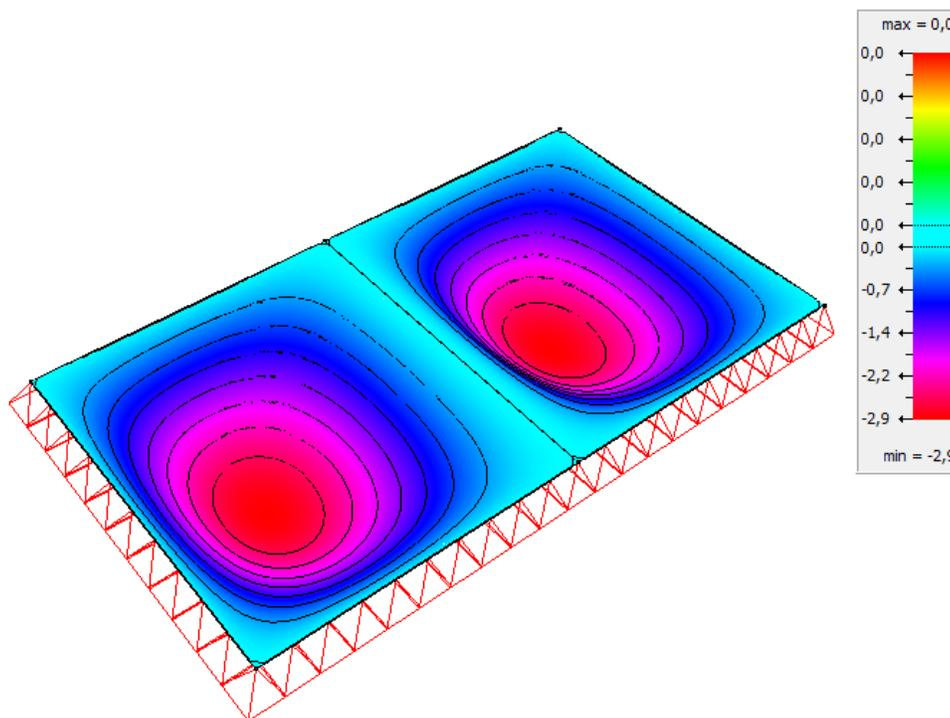
Figure 31: Deflections of floor panel - *Diamonds* (dimensions in mm) (Tine Lanssens and Charlot Tanghe) (BuildSoft)
