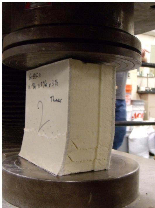
Figure 1-9 Compression test configuration with failed sample
