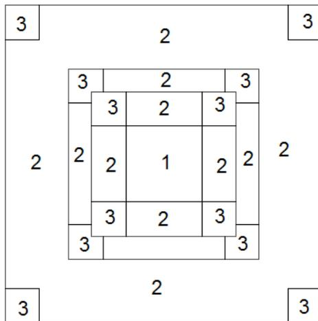
Figure 7: Wind Load Areas of the Solatrium roof
