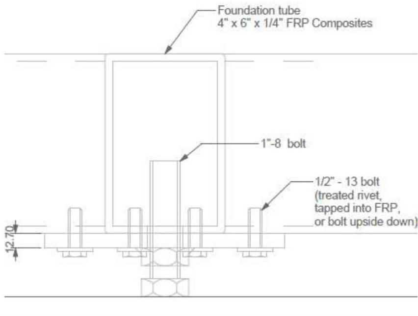
Figure 43: Support at the other nodes of the foundation grid (dimensions in mm) (BIM Report submitted to SD China 2013 by Team BEMANY on 3/6/2013)
