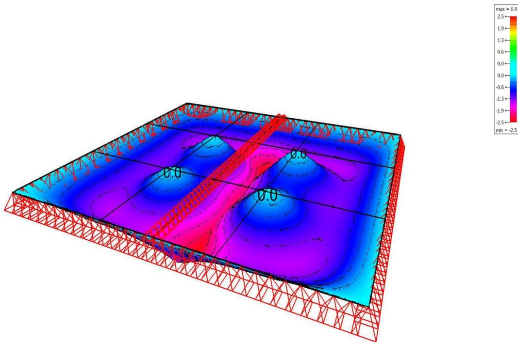
Figure 10: Deflection of the FEA Diamonds 2012 model with in four strut system (LC 1) (dimensions in mm) (BuildSoft)
