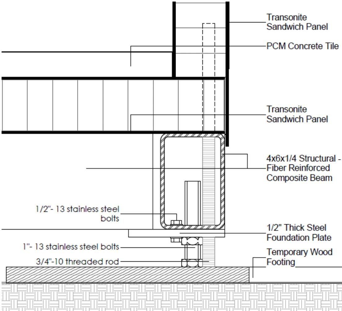
Figure 32 Floor connection diagram (BIM Report submitted to SD China 2013 by Team BEMANY on 3/6/2013)
