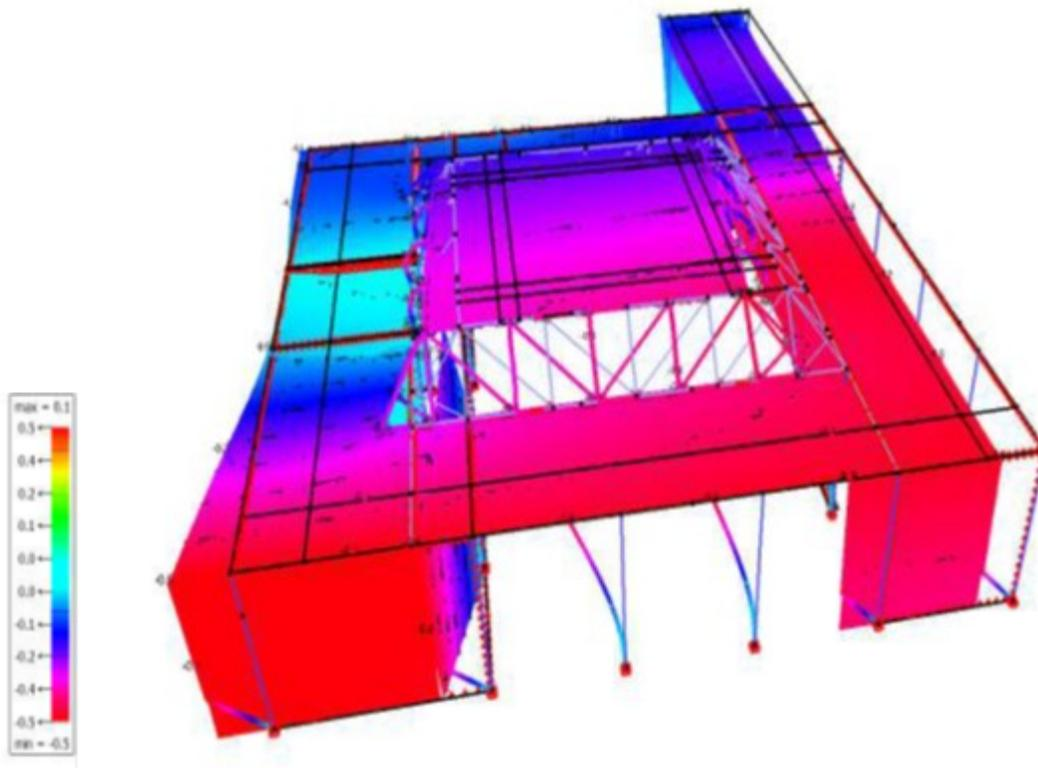
Figure 47 Seismic deflection in mm (loading applied east to west) (BuildSoft)
