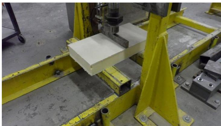
Figure 1-2 Creative Pultrusions Shear Test
