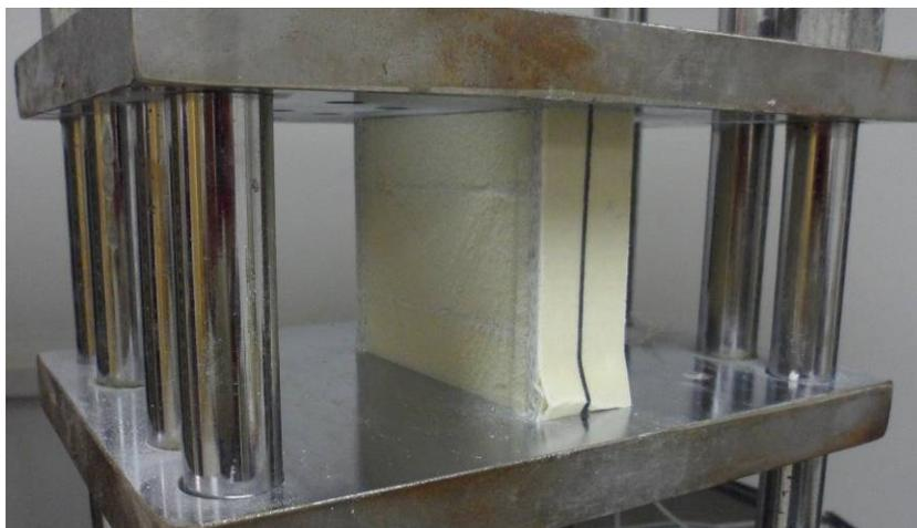
Figure 1-5 Creative Pultrusions InPlane Compression configuration and failed test specimen
