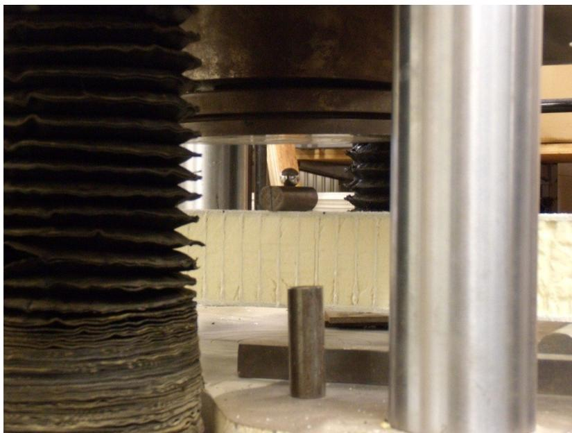
Figure 1-12 Long Beam 3 point bending test configuration
