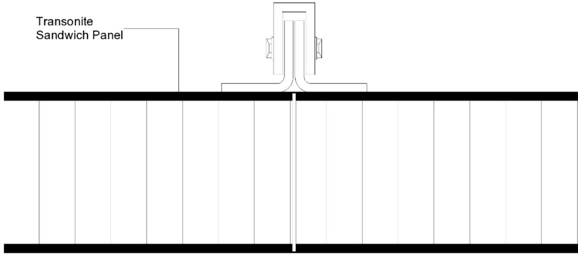
Figure 11: Detailed design of the seam between the Transonite™ atrium roof panels (BIM Report submitted to SD China 2013 by Team BEMANY on 3/6/2013)
