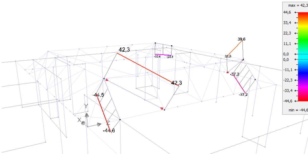
Figure 19: The 5 most axial loaded bars (loads in kN) (Thomas Tassignon) (BuildSoft)
