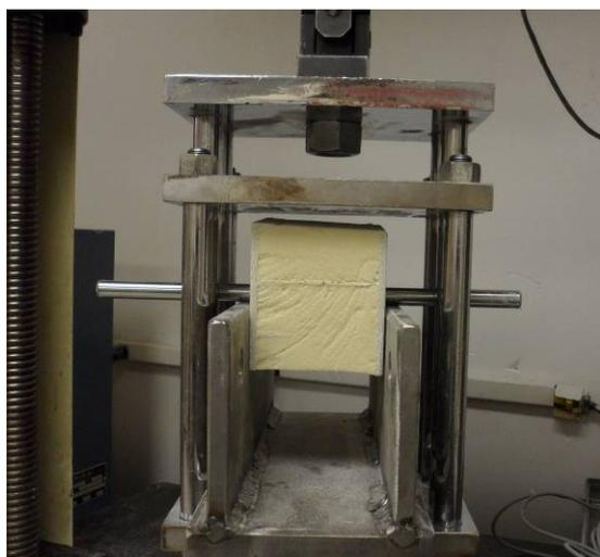
Figure 1-3 Creative Pltrusions Pin Bearing test configuration
