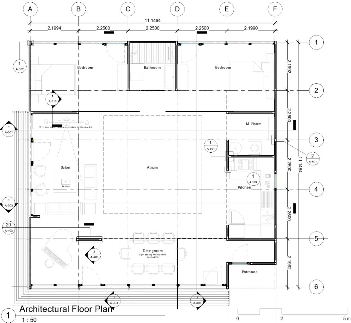
Figure 1 Interior Design Plan of the Solatrium (all units in meters) (BIM Report submitted to SD China 2013 by Team BEMANY on 3/6/2013)
