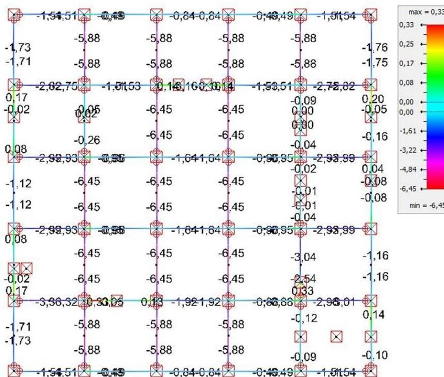
Figure 41: Deflections in the foundation tubes (in mm) (Tine Lanssens and Charlot Tanghe) (BuildSoft)
