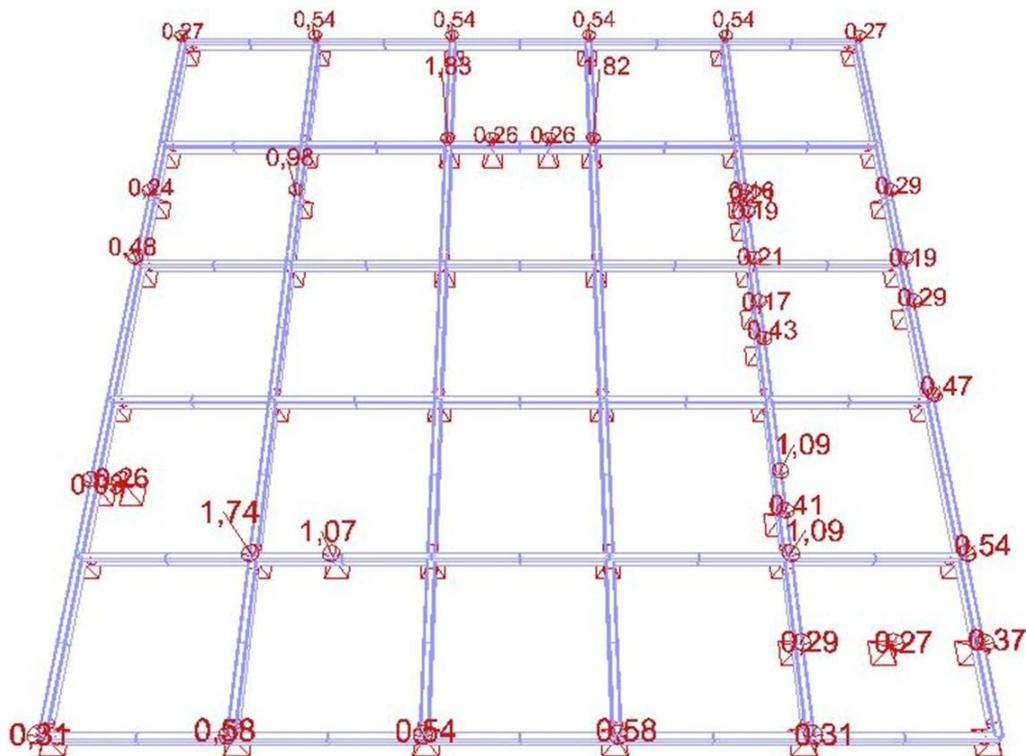
Figure 36: Point loads caused by the weight of the flat roof (without any load modifier) (loads in kN) (Tine Lanssens and Charlot Tanghe) (BuildSoft)
