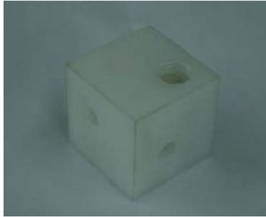
Figure 29 High Density Plastic Connection Cube (BIM Report submitted to SD China 2013 by Team BEMANY on 3/6/2013)
