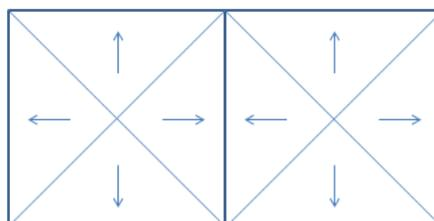
Figure 38: Triangular loading areas (outer beams and inner beams) (Tine Lanssens and Charlot Tanghe) (BuildSoft)
