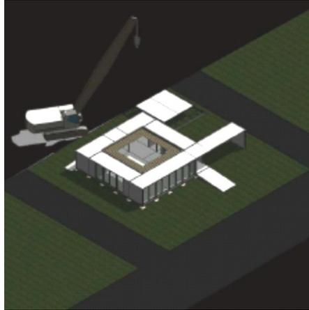
Figure 59 Rendering of the site after the roof places had been placed (BIM Report submitted to SD China 2013 by Team BEMANY on 3/6/2013)
