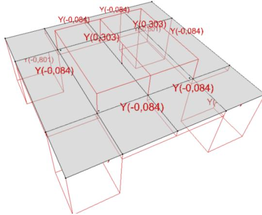
Figure 15: Wind loading distribution for upward lift loading (LC 2b) (loads in kN/m²) (BuildSoft)
