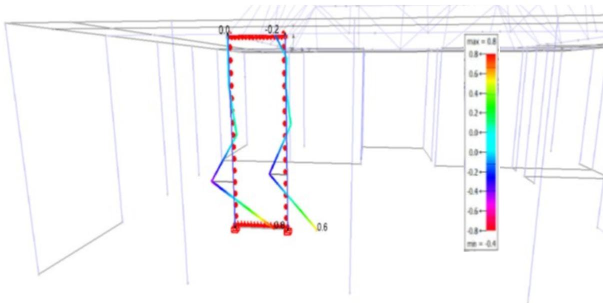
Figure 48 Moment caused by Seismic loading in KNm (BuildSoft)
