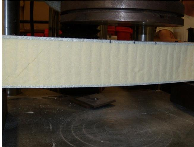
Figure 1-14 Long Beam after undergoing 3 point bending
