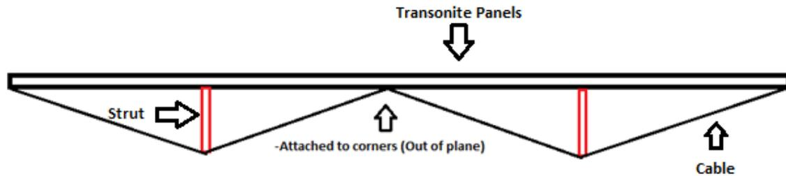
Figure 8: Diagonal section view of the roof and four strut cable stayed trusses
