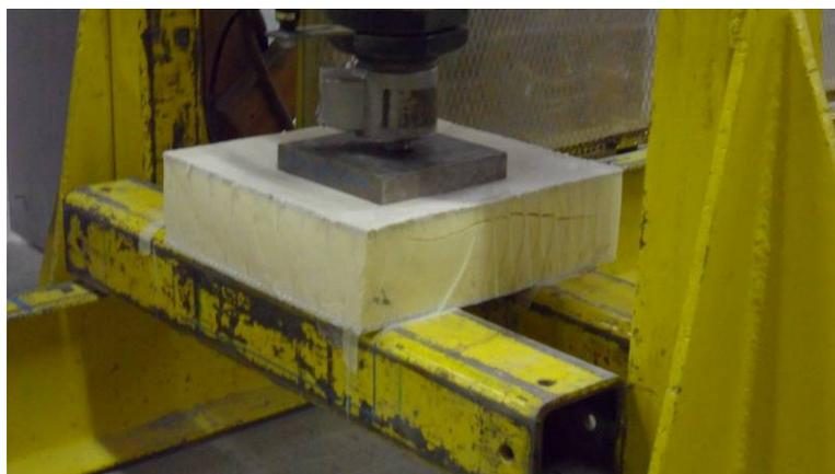
Figure 1-6 Creative Pultrusions 6" footprint configuration and Failed Sample
