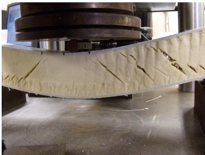
Figure 1-13 Long bending 3 point under loading.
