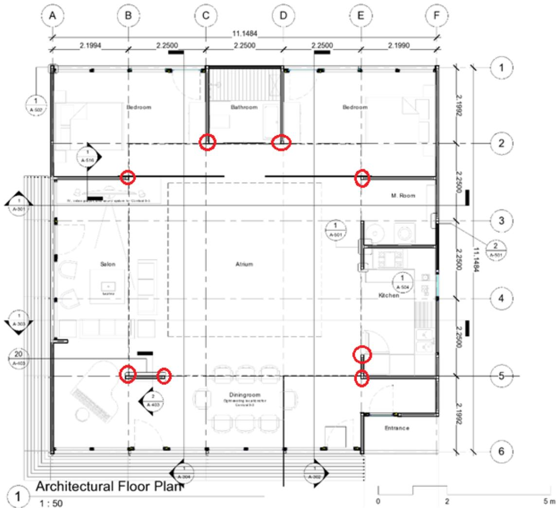
Figure 28 Floor plan with reinforced columns indicated by red circles (BIM Report submitted to SD China 2013 by Team BEMANY on 3/6/2013)
