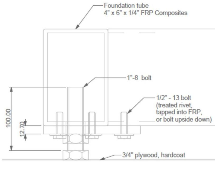
Figure 42: Support at the edge of the foundation grid (dimensions in mm) (BIM Report submitted to SD China 2013 by Team BEMANY on 3/6/2013)
