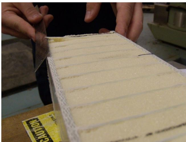
Figure 1-17 a failed connection point of the glass fibers and the FRP skin
