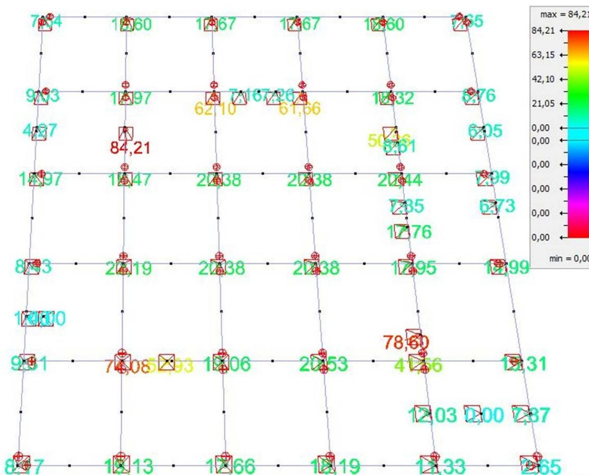
Figure 44: Vertical reaction forces on the foundation grid (reactions in kN) (Tine Lanssens and Charlot Tanghe) (BuildSoft)
