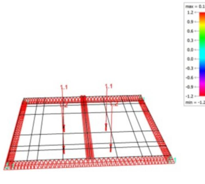
Figure 17: Reaction forces given by the model on the four struts (LC 2b) (forces in kN) (BuildSoft)
