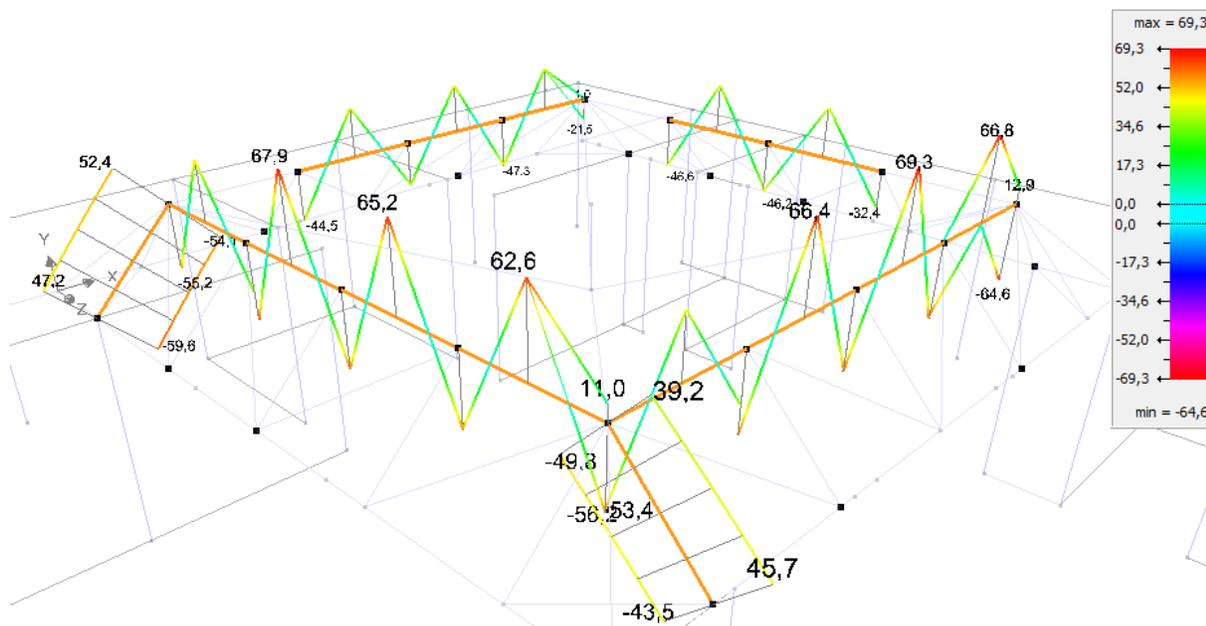
Figure 22: 15 maximal stresses in square tubes (stresses in kN/mm<sup>2</sup>) (Thomas Tassignon) (BuildSoft)
