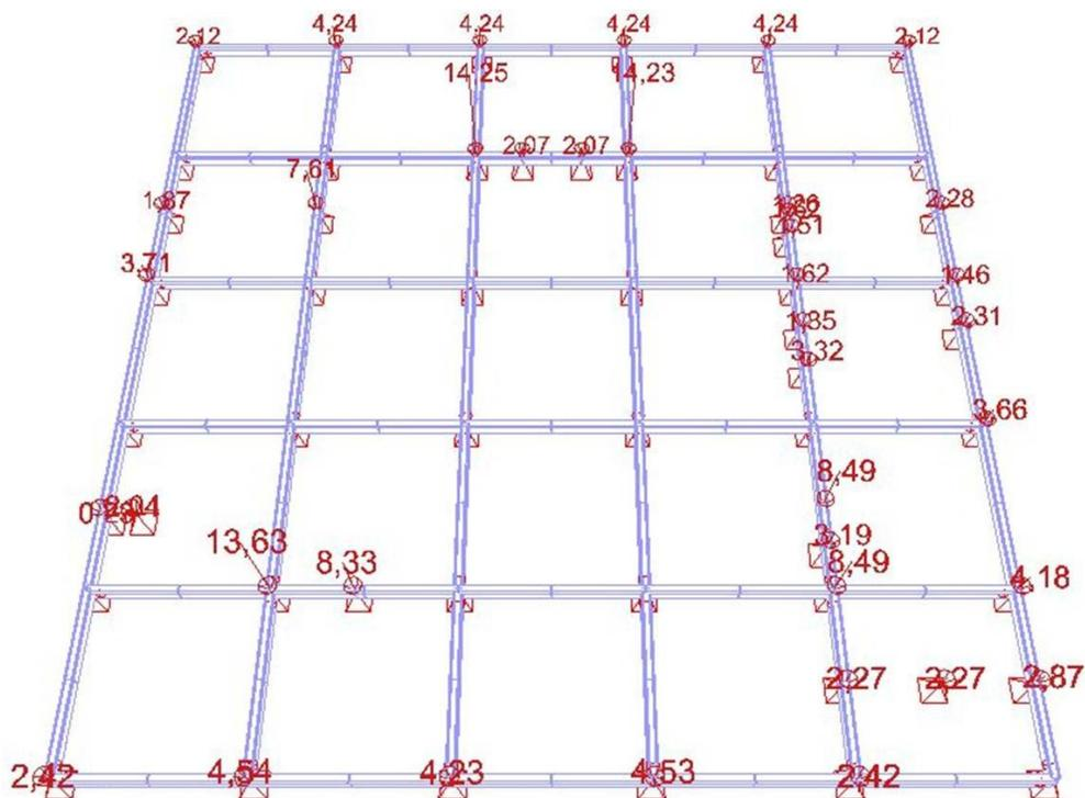
Figure 35: Point loads caused by the snow on the flat roof (without any load modifier) (loads in kN) (Tine Lanssens and Charlot Tanghe) (BuildSoft)
