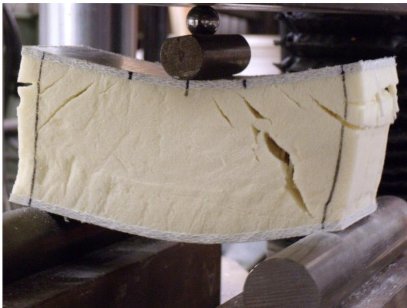
Figure 1-10 short Beam testing configuration with sample under loading
