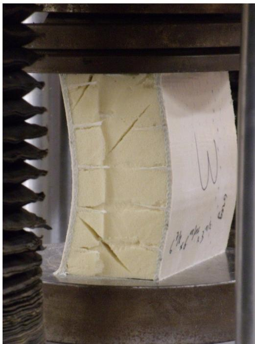
Figure 1-16 Compression testing sample under loading showing the shear cracking of the foam.
