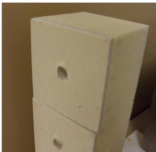
Figure 1-4 Creative Pultrusions Pin Bearing Failed Test Samples
