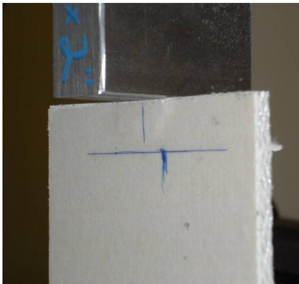
Figure 1-8 CREATIVE PULTRUSIONS EDGE LOADING failed sample
