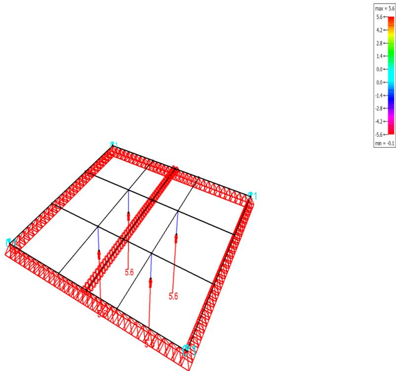
Figure 12: Reaction forces given by the FEA model on the four struts (LC 1) (forces in kN) (BuildSoft)
