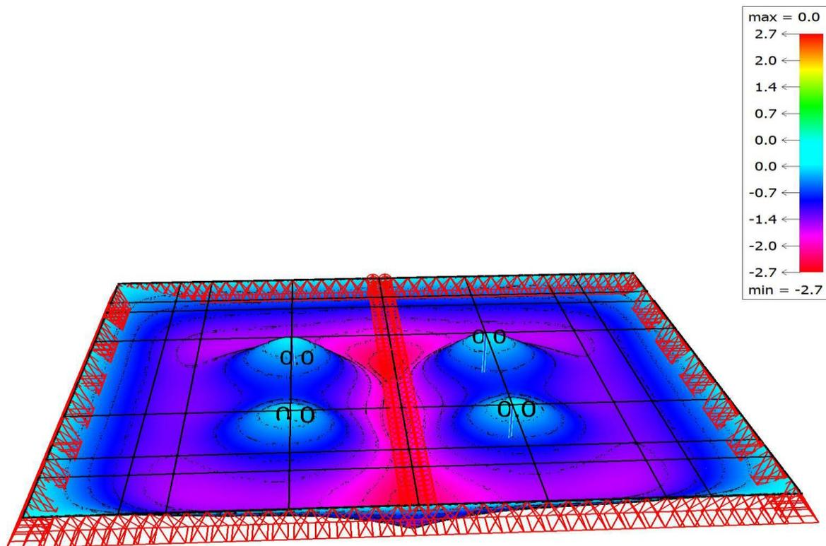
Figure 13: Deflections of the FEA model with 5 struts (LC 2a) (dimensions in mm) (BuildSoft)
