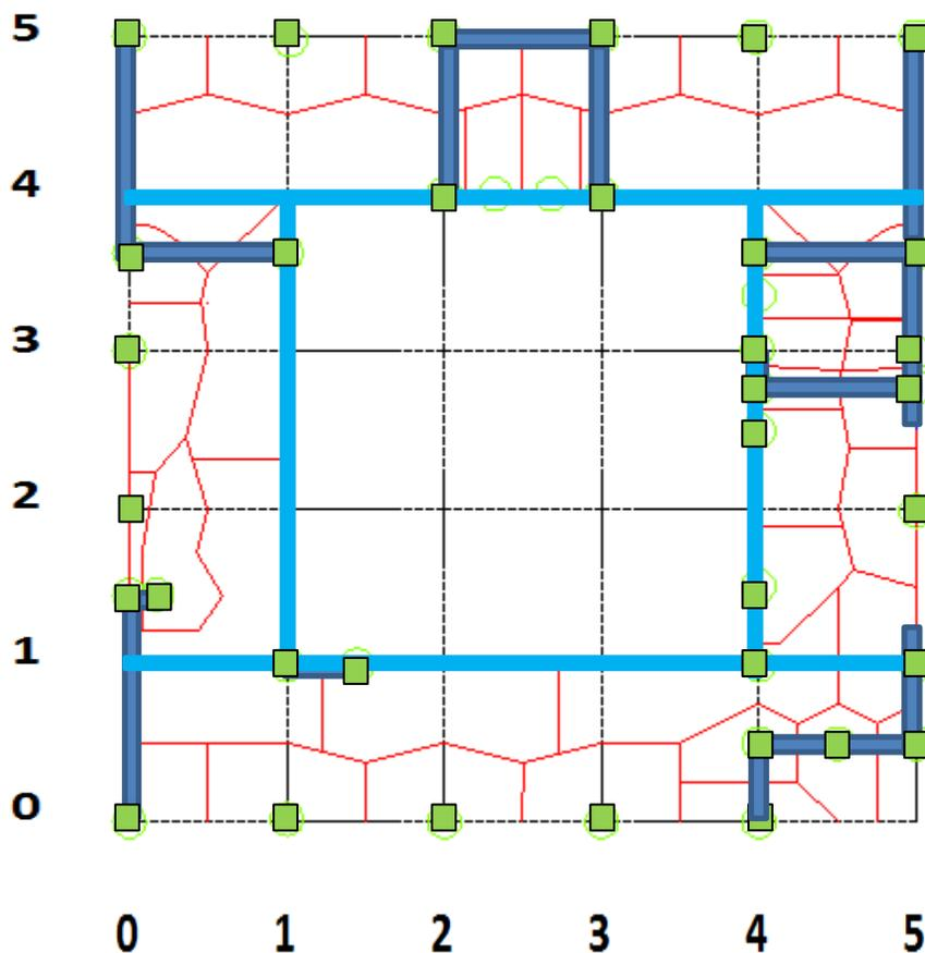
Figure 27: Tributary areas flat roof (blue represents walls, light blue represents beams, green represents columns)
