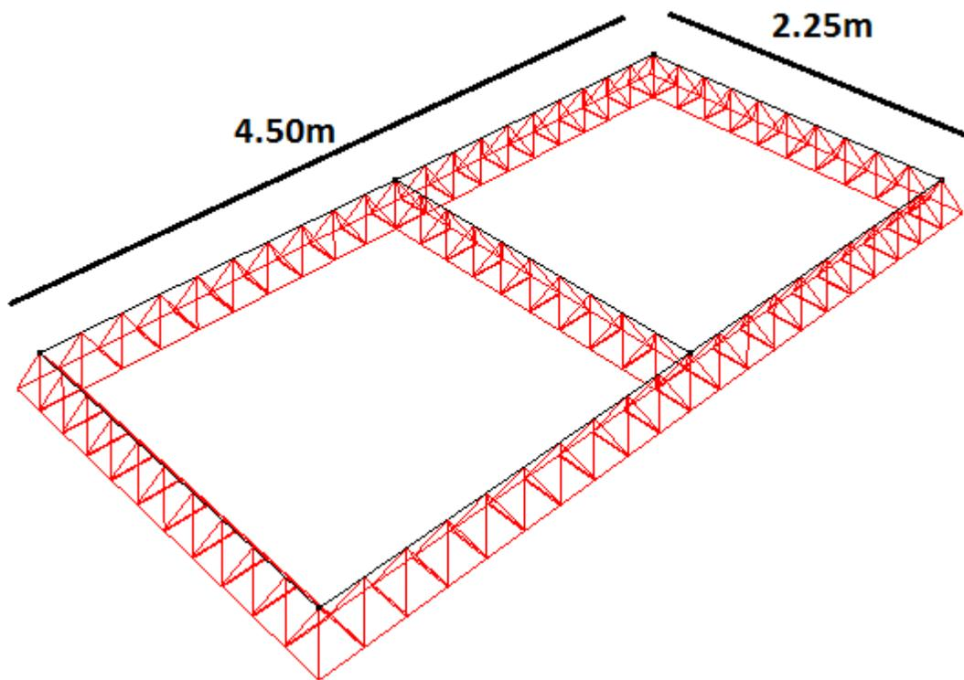
Figure 30: Supports of floor panel (2.25m x 4.50m) (Tine Lanssens and Charlot Tanghe) (BuildSoft)
