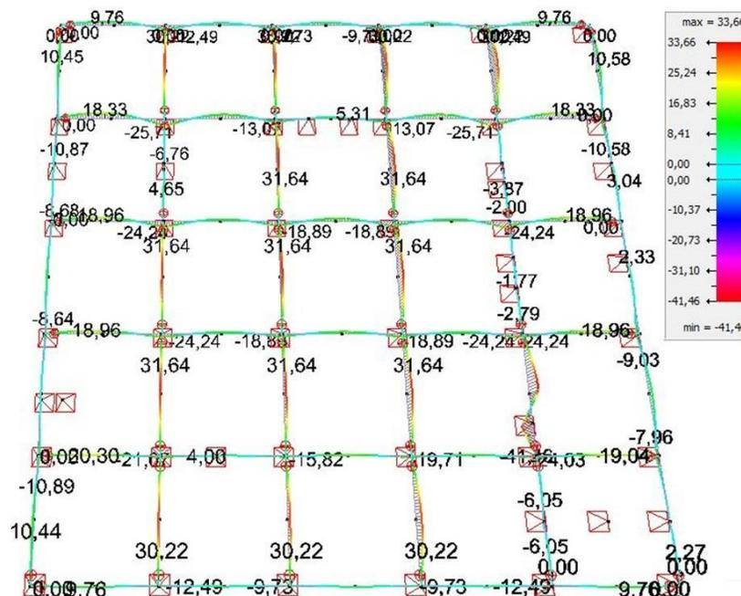
Figure 40: Normal stresses along the strong axis (in N/mm²) (Tine Lanssens and Charlot Tanghe) (BuildSoft)
