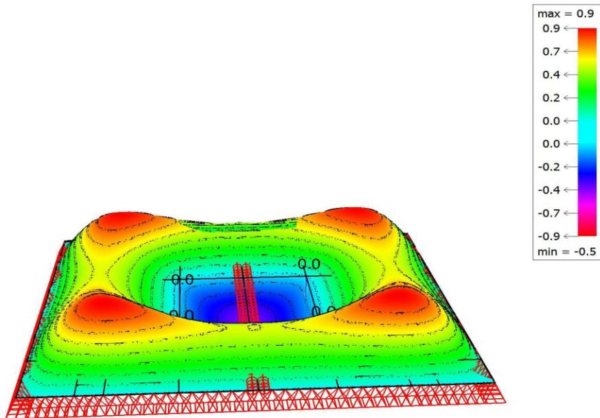
Figure 16: Deflections of the FEA model with 4 struts (LC 2b) (dimensions in mm) (BuildSoft)
