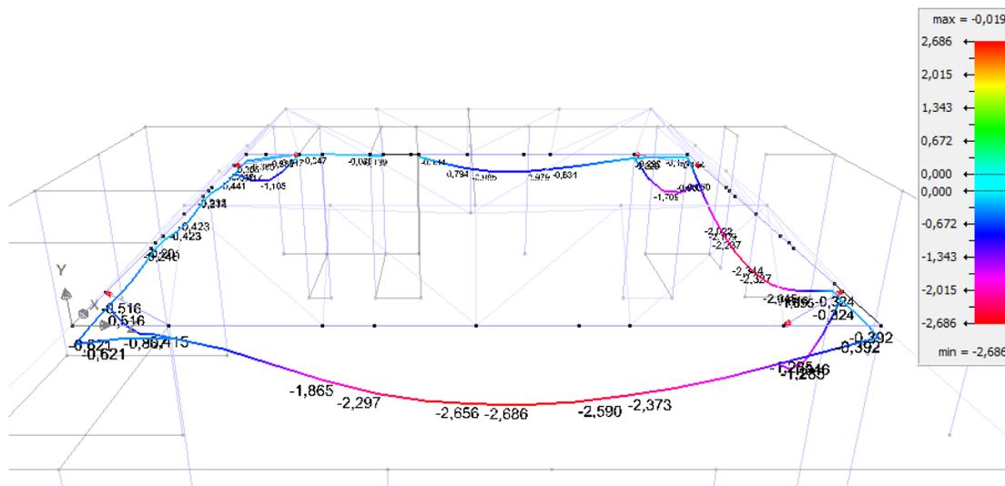
Figure 26: Deflections in bottom chord of atrium truss (dimensions in mm) (Thomas Tassignon) (BuildSoft)
