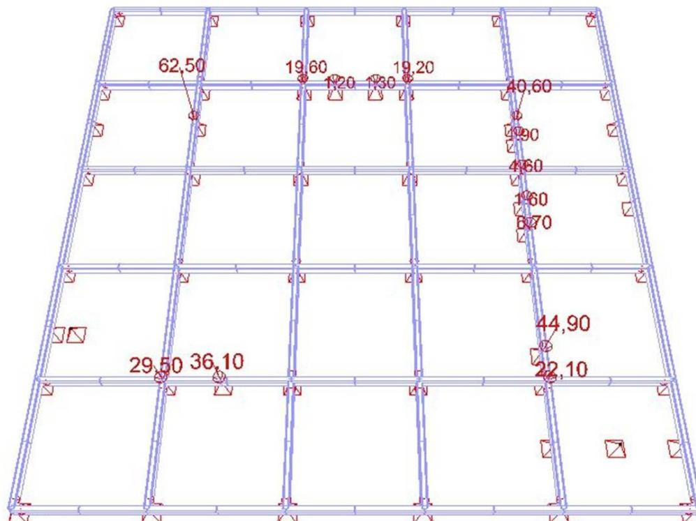
Figure 37: Point loads caused by the loads on the atrium roof (using the load combination 1.2 Dead Weight and 1.6 Snow load) (loads in kN) (Tine Lanssens and Charlot Tanghe) (BuildSoft)
