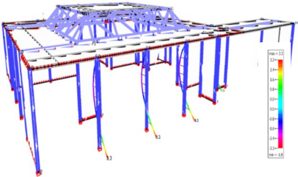
Figure 45 Max moments caused by Horizontal wind loading in KNm (BuildSoft)
