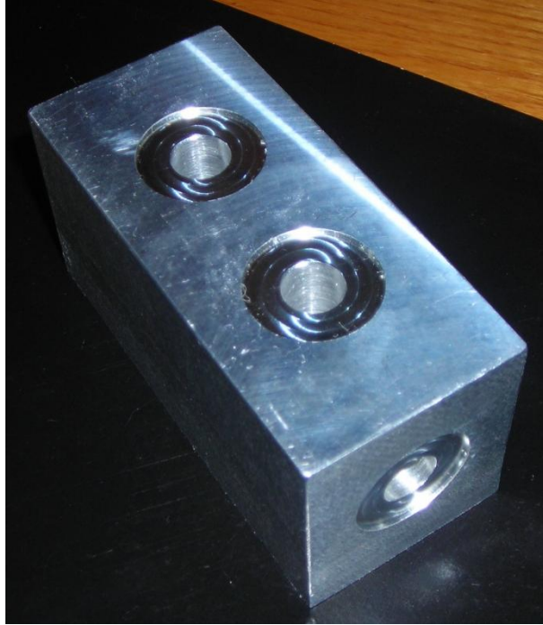
Figure 37 Manifold Block from Original Strategy
