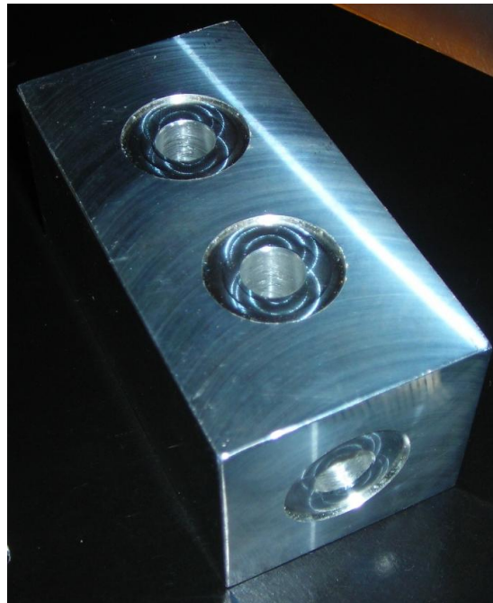
Figure 38 Manifold Block from Improved Strategy
