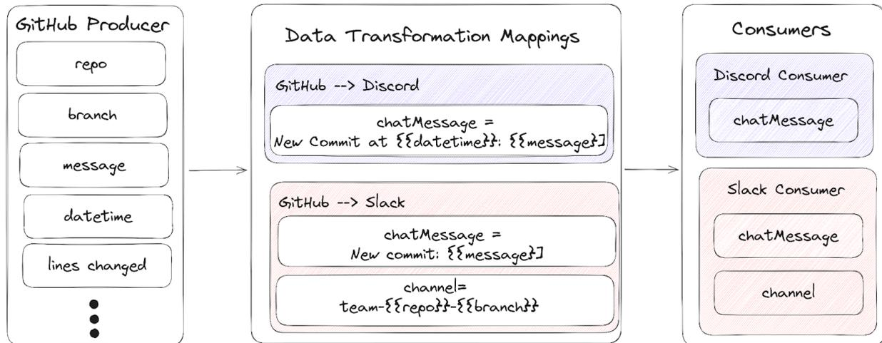
Figure 2. Data transformation from Producer to Consumer
