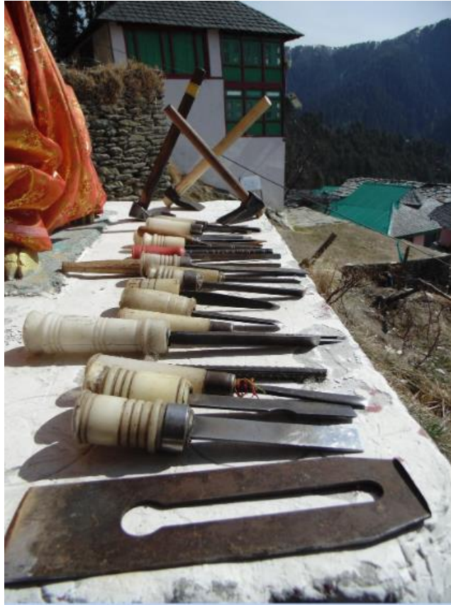
Figure 18: Contemporary tools from wood carvers of the Thaiyi caste in Somgad. From front-to-back: planer, varying chisels, splitter/mallet.
