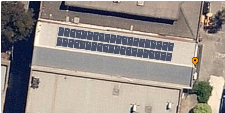
Figure 5 - North Facing Panels on a Slanted Roof (NearMap)
