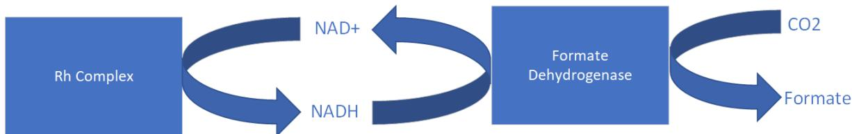
*Figure 4: Flow Cell Diagram showing the flow of electrons and the reduction of  $\text{CO}_2$  to formate as a product and the regeneration of NADH via immobilized Rh complex.*
