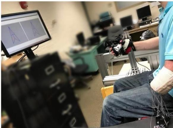
Fig. 7.1. Experimental apparatus. Subjects (limb-absent subject shown) sat in a chair with each able hand secured into force measurement devices, facing the computer screen which displayed a target and real-time force/moment feedback.
