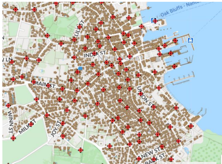
Figure 7. Map of fire hydrants in downtown Nantucket, Massachusetts. The red and brown symbols indicate fire hydrants and houses, respectively.
