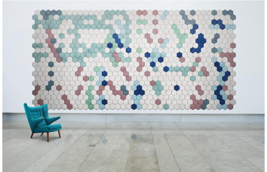
**Figure 19:** An example of a decorative sound absorbing wall (Soundproofing, 2020).
