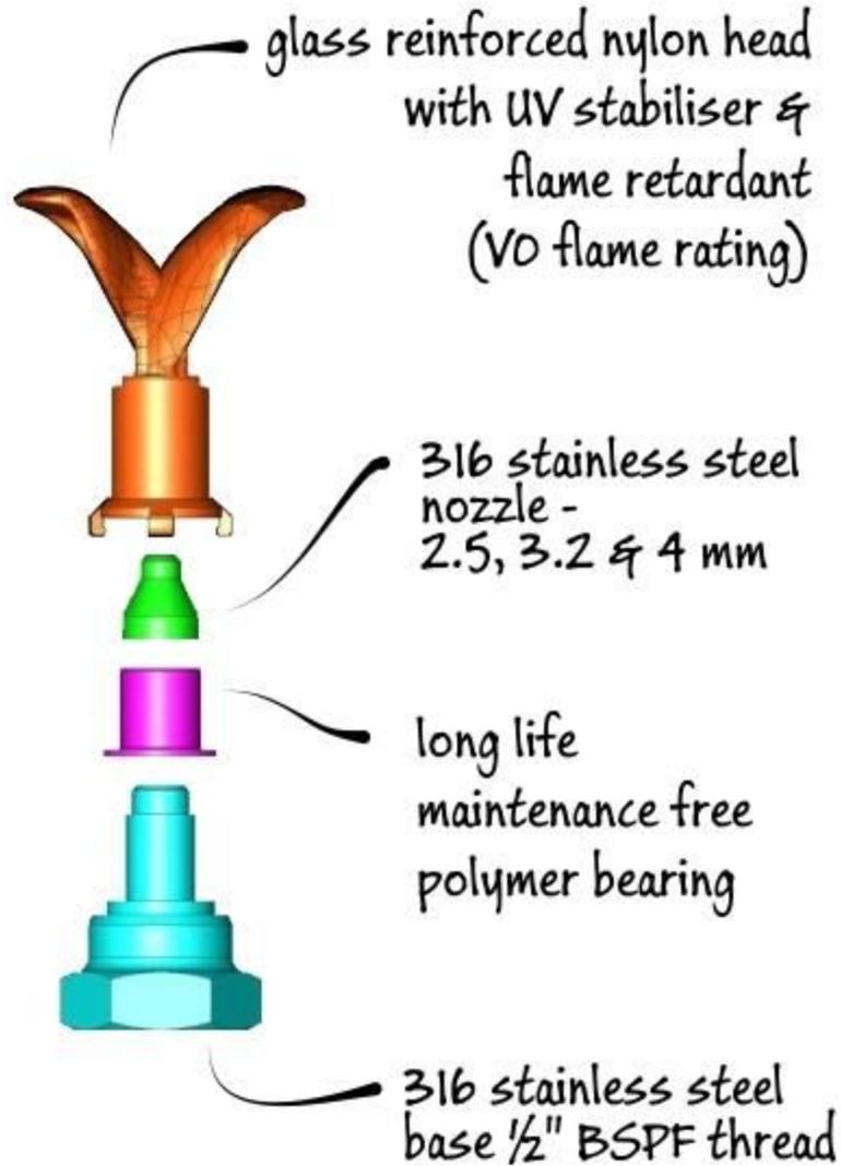
*Figure 10: A Platypus sprinkler heads deconstructed to show detail [n]*
