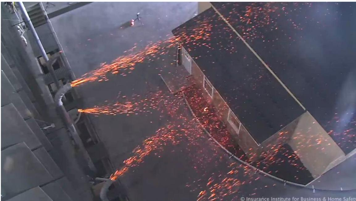
*Figure 2: A 2013 IBHS test with firebrand ember generators to simulate a WUI wind storm igniting a residential building [b].*
