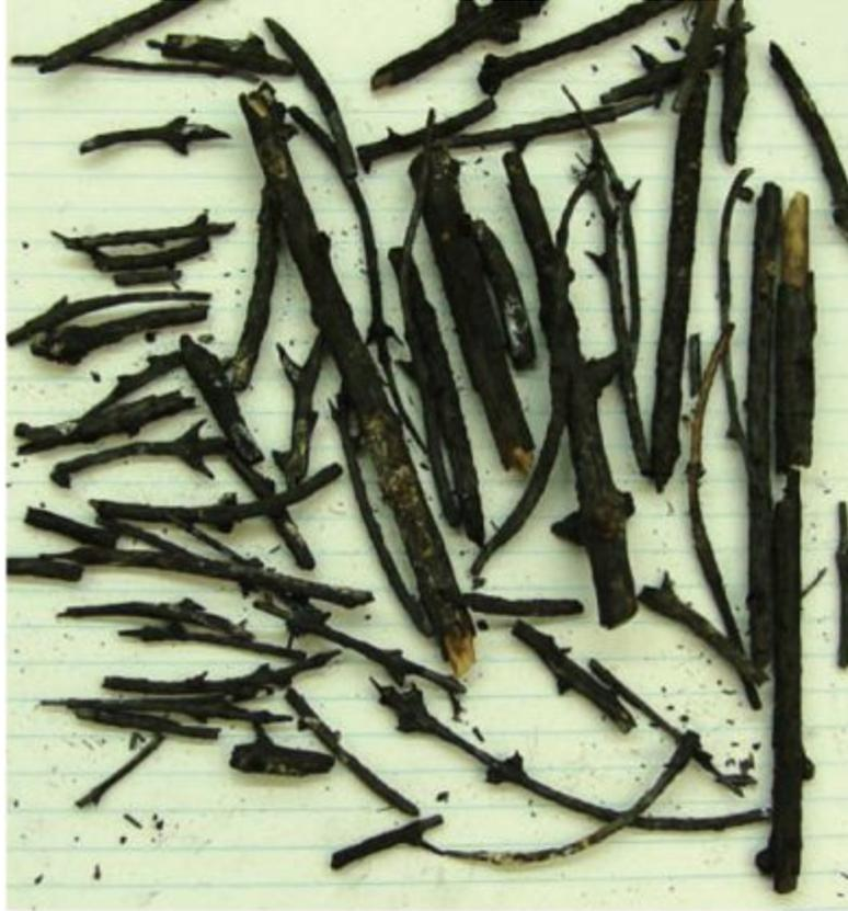
*Figure 4: Firebrands from a 5.2-meter tall tree with a moisture content of 20% (Manzello, 2017) [d]*
