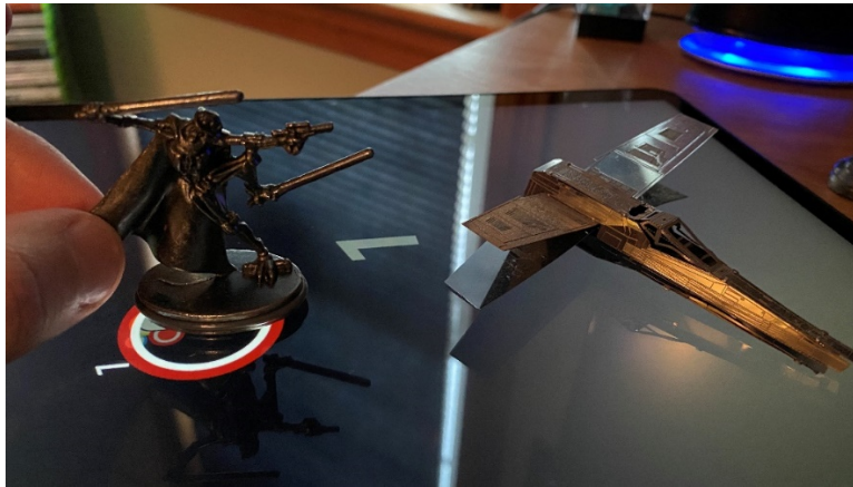
Figure 15. The pewter figure is easily sensed while the steel one is not [Source: Author].
