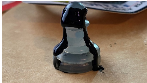
Figure 19. A Chess pawn covered with conductive ink used during Roll [Source: Author].
