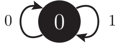
Figure 3.2: The Markov chain of the status update system regarding \Delta_i(t) for case RND_NR. Link \ell = 0 corresponds to a successfully delivered packet for \mathcal{S}_i . Link \ell = 1 corresponds to an unsuccessfully delivered packet for \mathcal{S}_i as well a successful or unsuccessful packet from any other source.
