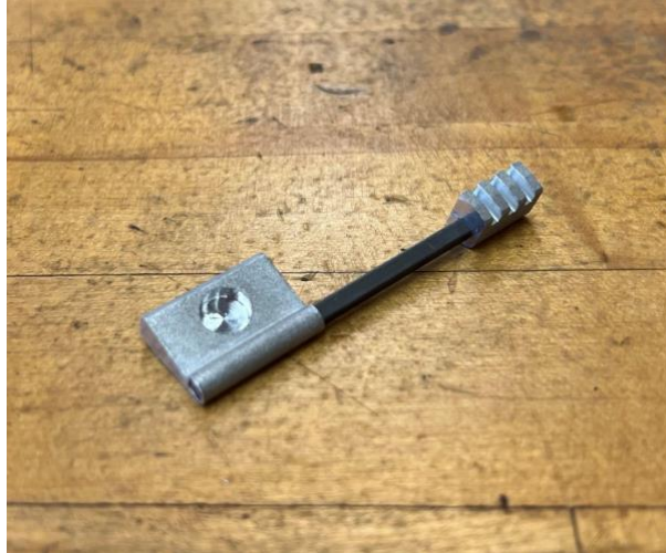
Figure 82: Key Handle with Rod Pressed into Place and Locking Key Attached
