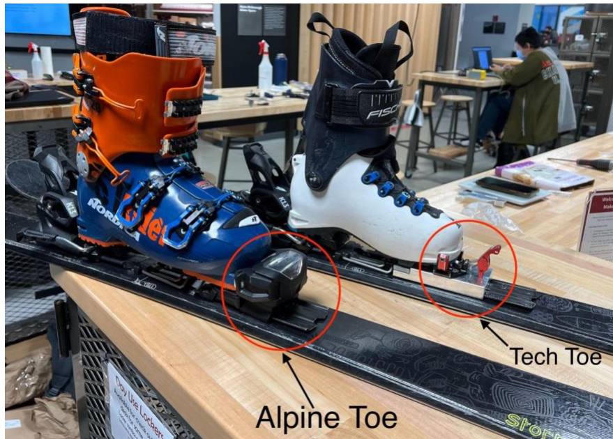
Figure 92: Binding System Mounted to Ski
