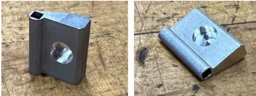
Figure 75: Two Perspectives of the Final Machined Key Handle
