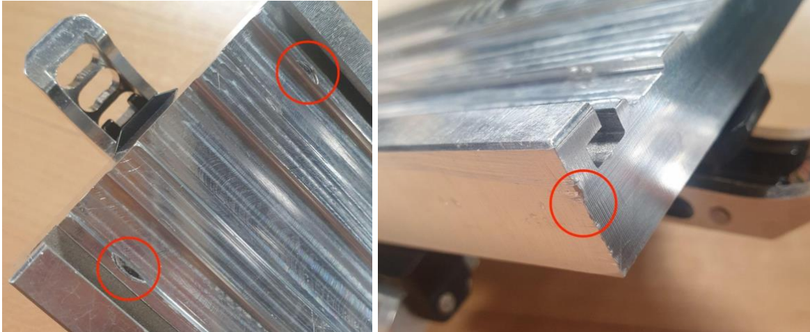
Figure 94: Two Points of Cosmetic Wear on Tech Toe Plate
