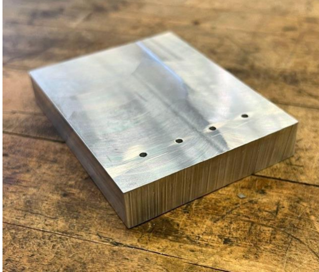
Figures 65: Stock Material for Locking Key After First Two Programs
