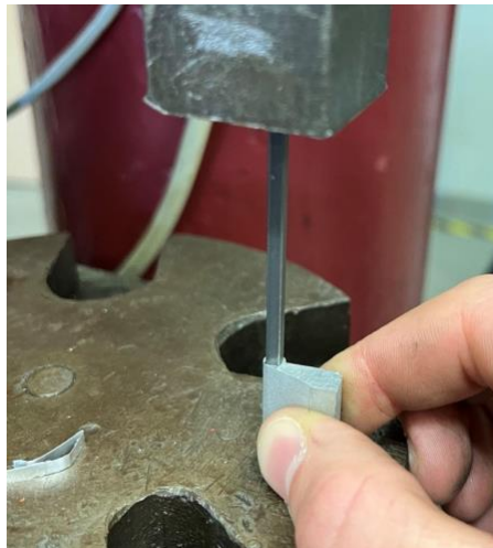
Figure 81: Pressing the Rod into the Key Handle Using the Arbor Press (image shown for demonstration only)
