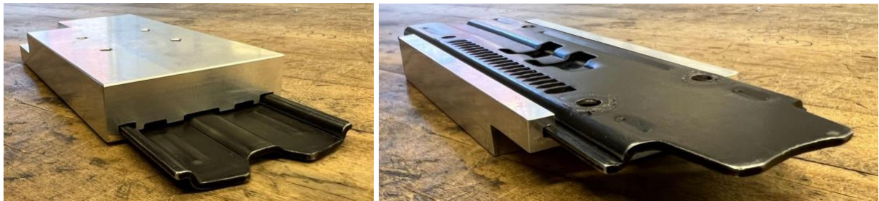
Figure 78: Two Perspectives of the Fitment Between Tech Toe Plate and Tyrolia Rail
