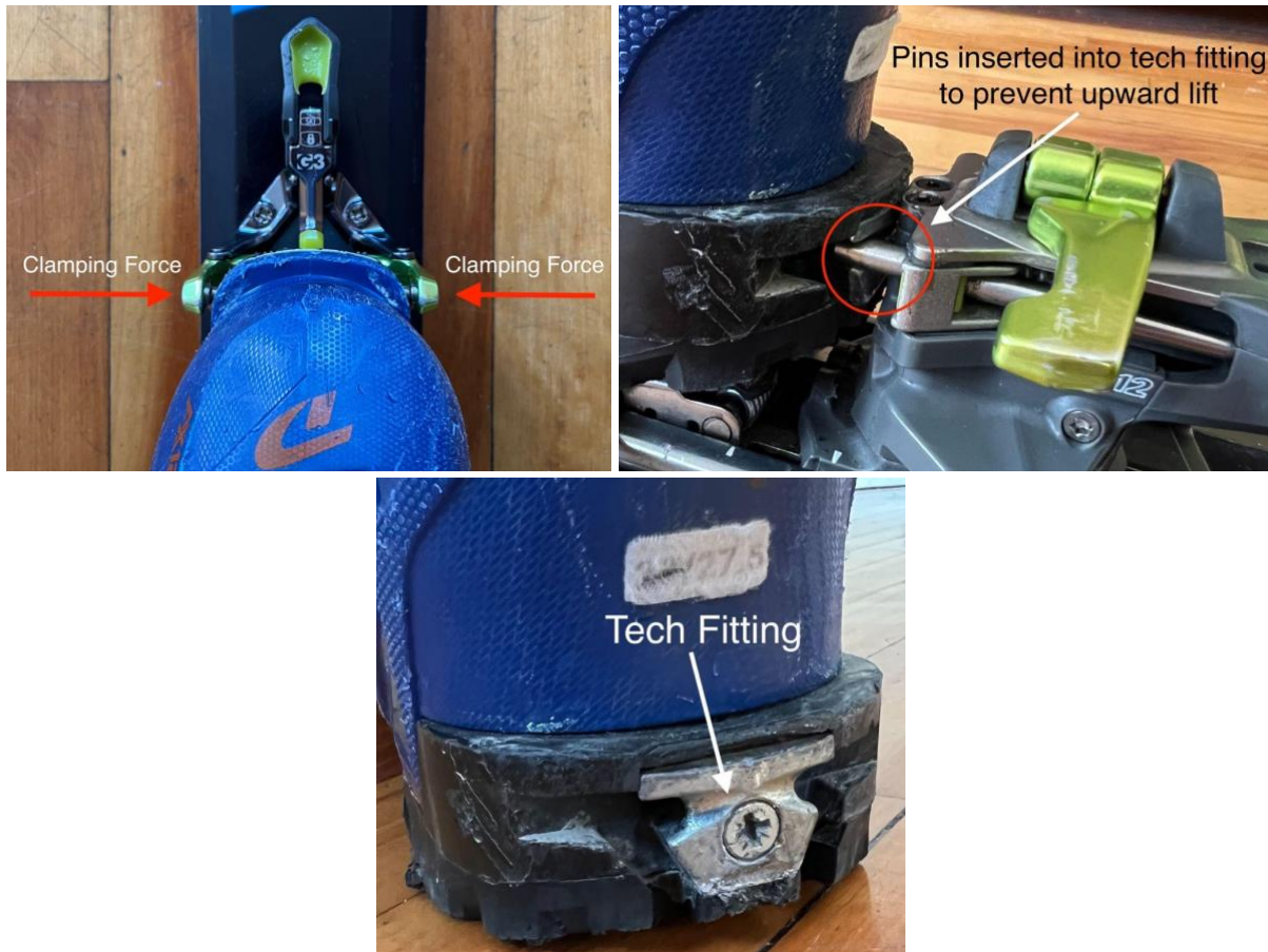
Figure 10: Different Views of Clamping Mechanism of a Tech Binding
