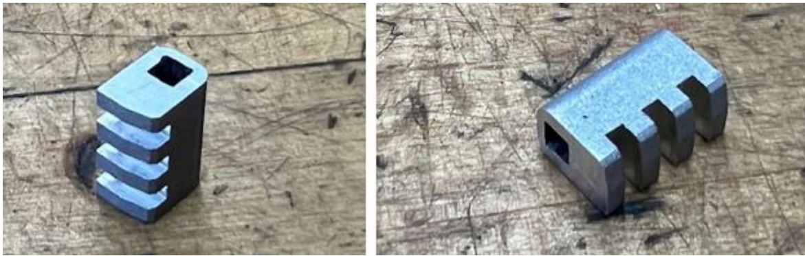
Figure 70: Two Perspectives of the Final Machined Locking Key
