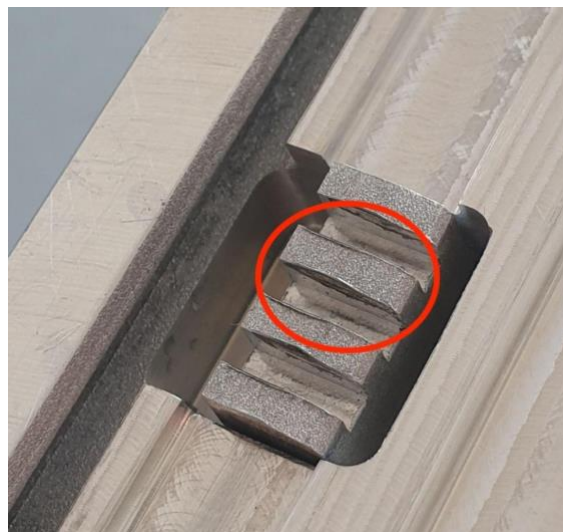
Figure 95: Wear on Locking Key Teeth
