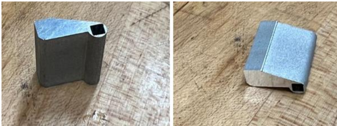
Figure 74: Two Perspectives of the Key Handle After the Wire EDM Operations
