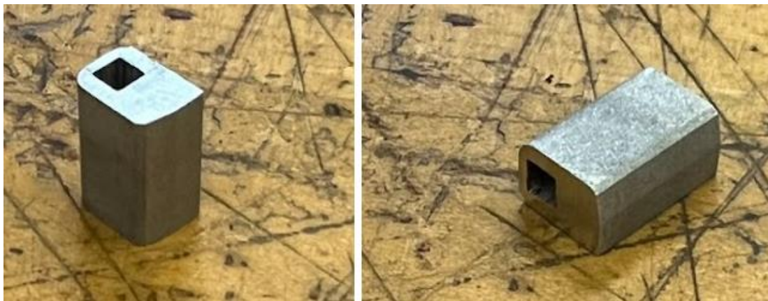
Figure 68: Two Perspectives of the Locking Key After the Wire EDM Operations
