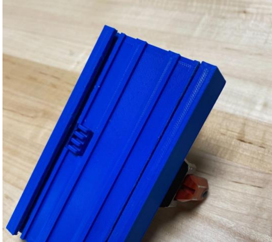
Figure 53: Underside of Tech Toe Plate with Rail Cutouts and Locking Key Mechanism
