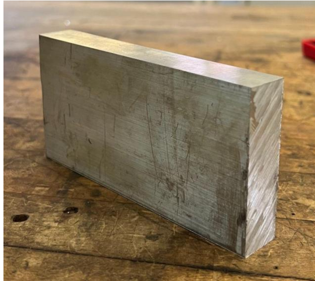
Figure 57: Progress After Initial Milling Operation
