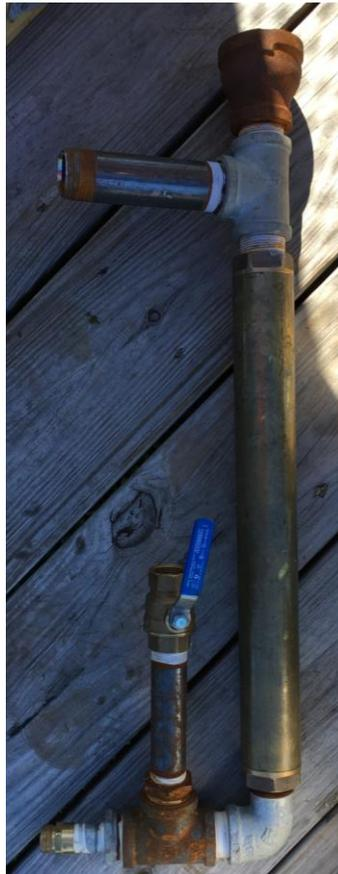
*Figure 35: Fill Point Assembly*
