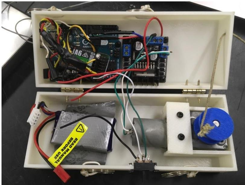
*Figure 34: Inside of Final Motor Box*
