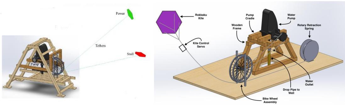
Figure 15: Two-Kite Retraction System vs Rotary Spring Retraction System
