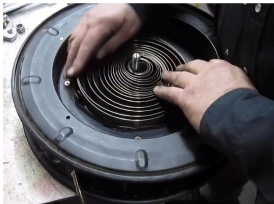
Figure 18: Inside a Linear Reel Spring
