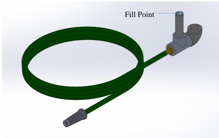
*Figure 31: Surface Pump Assembly CAD with Fill Point called out*
