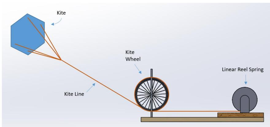
Figure 20: Kite Line Torque Transfer Method
