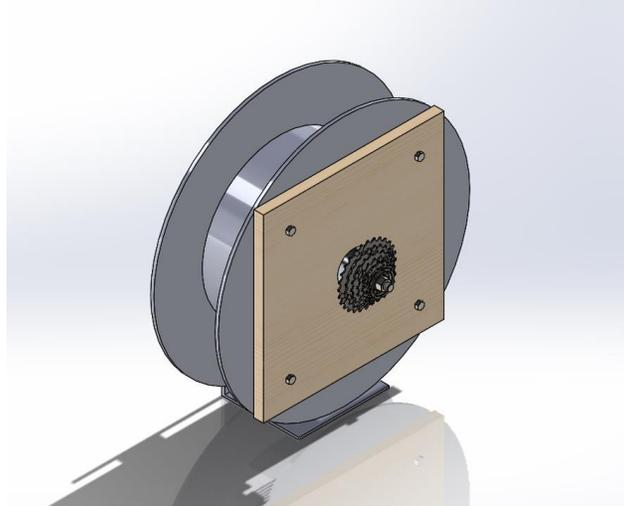
Figure 21: Rotary Spring with Gear Train
