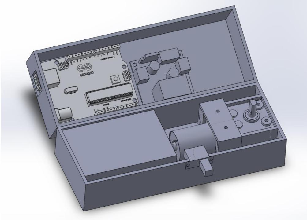
*Figure 14: Initial CAD of circuit organization in casing*
