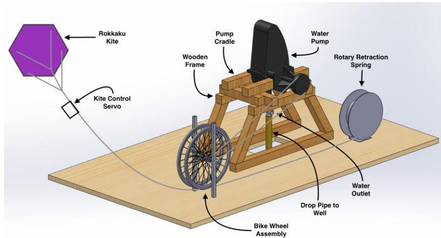
Figure 29: Complete CAD assembly of kite power system (excluding chain tensioner and kite wheel supports)
