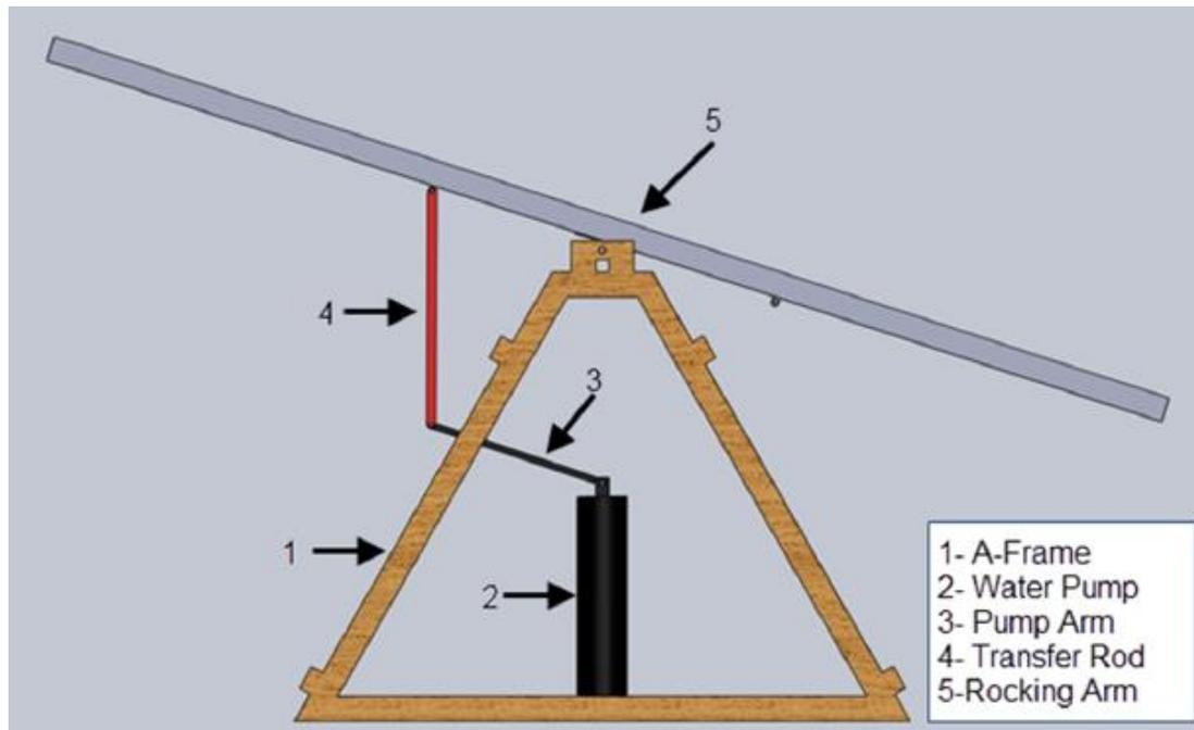
Figure 7: SolidWorks Model of Rocking Arm Design (Bartosik et al. 2012)
