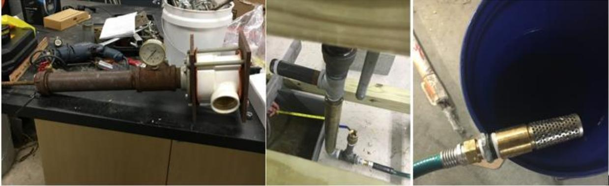
*Figure 30: Old pressure valve (left) versus new surface pumping system (center, right).*
