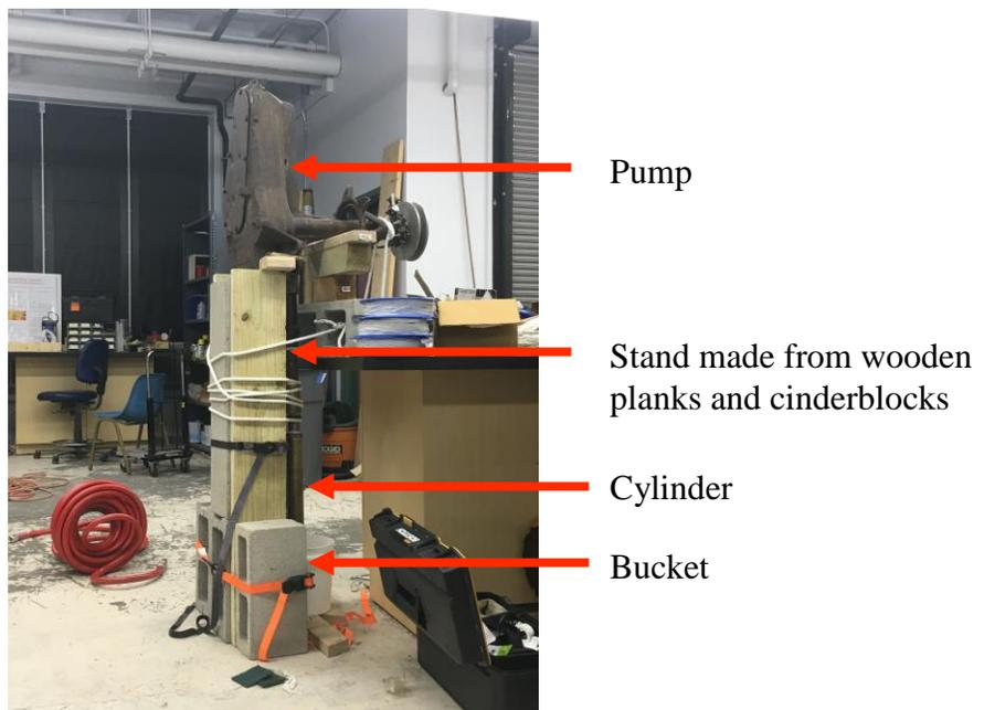
Figure 26: Reduced pump subsystem test setup
