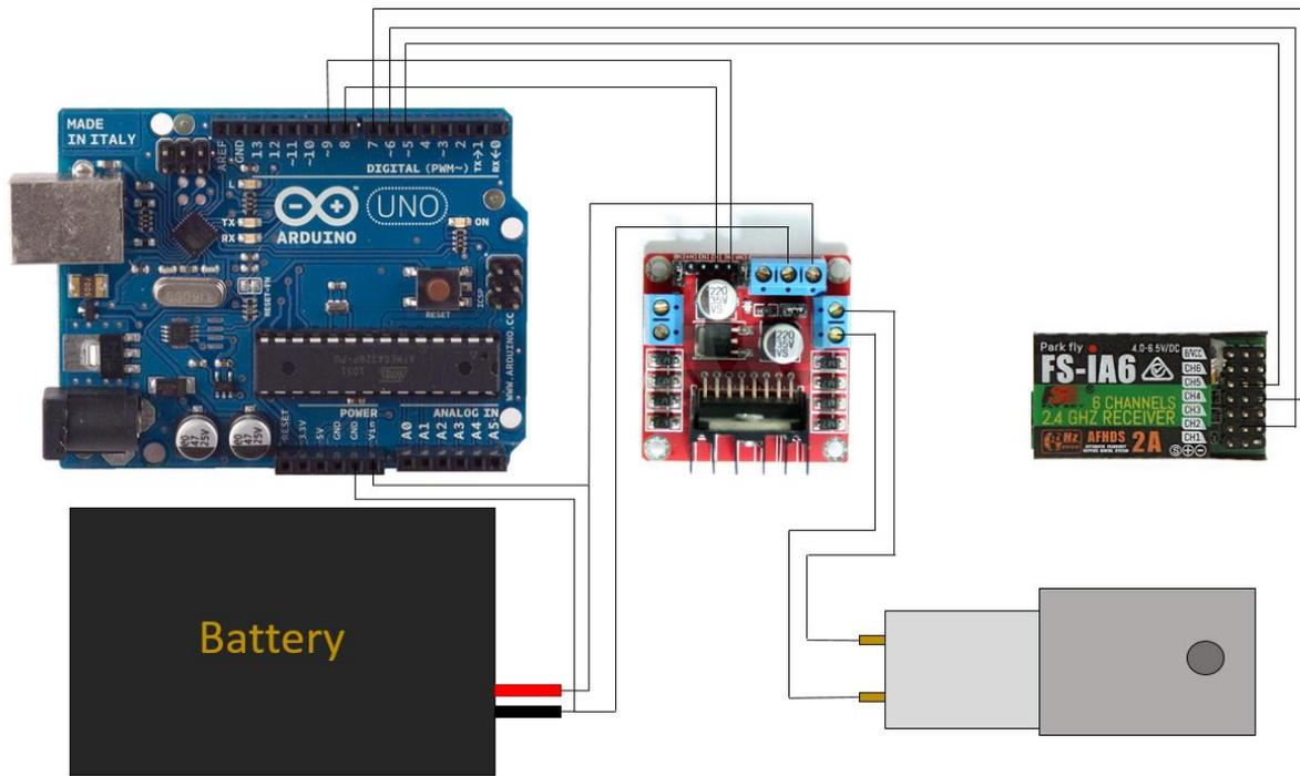
Figure 12: Circuit Diagram of Motor Configuration
