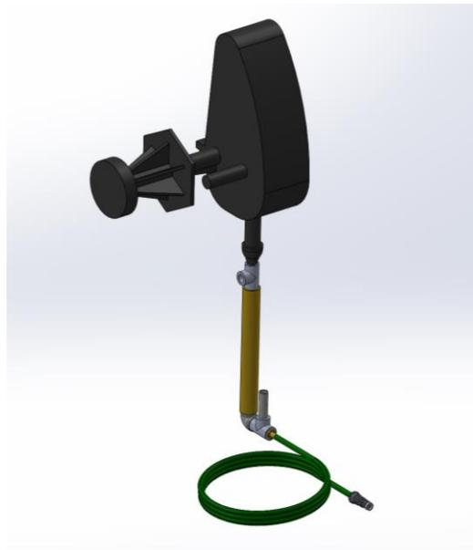
*Figure 32: Full pump assembly including surface pumping*
