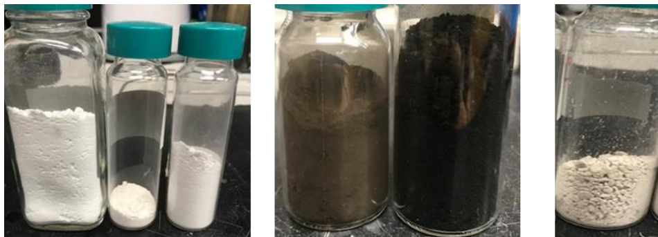
Figure D5-15. Photographs highlighting the difference in catalyst color from re-use. Photographs comparing the initial fresh HAP catalyst, the catalyst after in situ hydrothermal liquefaction and after ex situ hydrothermal liquefaction, related to catalyst characterization, Table 5-1 and Figure 5-2.
