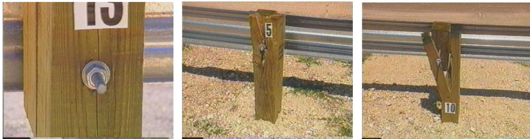
**Figure 2.12:** Posts split vertically during TTI test 404201-1 along pre-existing splits in posts. (32)
