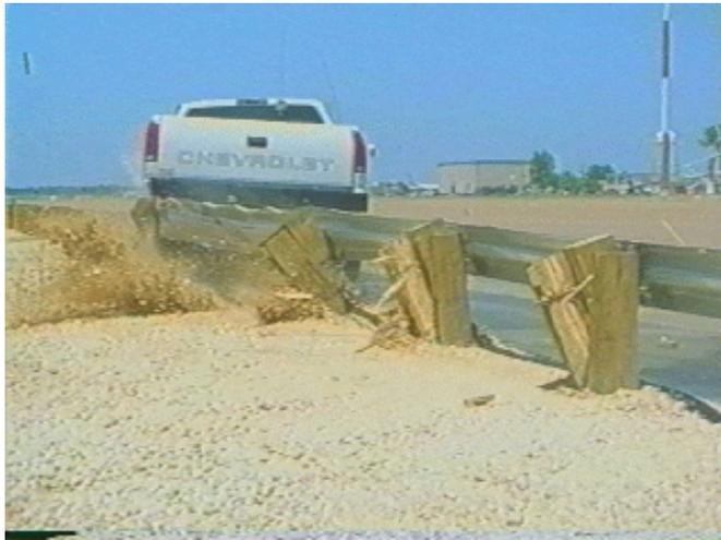
**Figure 2.11:** Guardrail damage in test TTI 404201-1.
