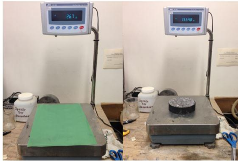
a. The specimen and “Corelok Bag” are weighed and recorded
