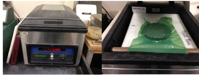
b. The specimen is sealed inside “Corelok Bag” using Corelok machine which is set to program 2.
