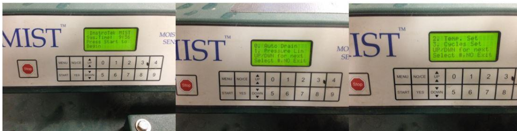
c. The parameters for which the specimens will be conditioned at can be set under menu in the MIST machine. MIST conditioning parameters: Temperature (25°C), Cycles (10,000), Pressure (30 psi)
