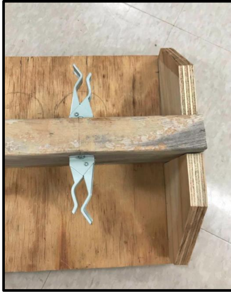
Figure 38: Attachment of the spring grips to the odor bank prototype.
