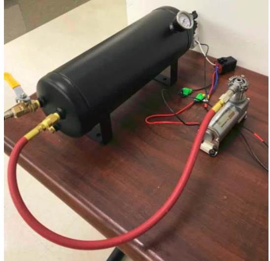
Figure 3B: Fully assembled compressor and air tank
