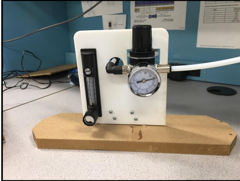
Figure 32: Flow control component mounting plate prototype. The flow meter is shown on the left and the pressure gauge is shown on the right.
