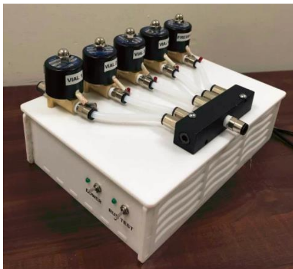
Figure 8B: Fully assembled power control box
