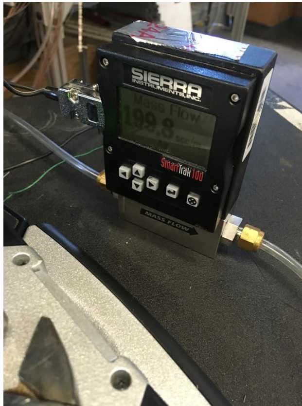
Figure 50: Mass flow meter and its display, which fluctuated around 200 cc/min. In the image the display reads 199.8 cc/min.
