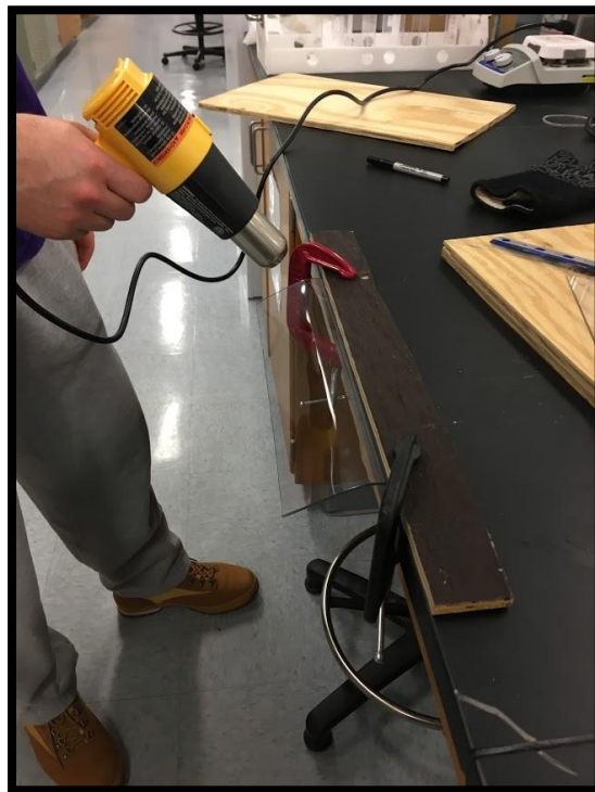
Figure 55: This image shows the process of heating and bending the Lexan to form the cover for the odor bank
