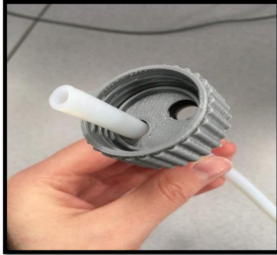
Figure 54: The custom-made 3D printed centrifuge tube caps with inserted O-rings
