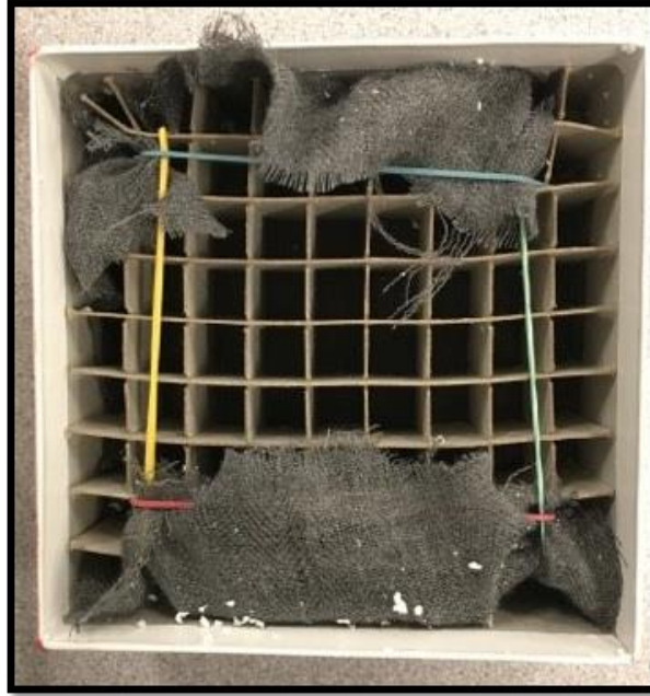
Figure 41: The team's prototype of the filter to house in the adapter, constructed out of cardboard, cloth, and rubber bands.
