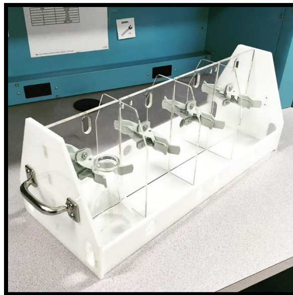
Figure 53: The laser-cut and assembled acrylic odor bank with handles
