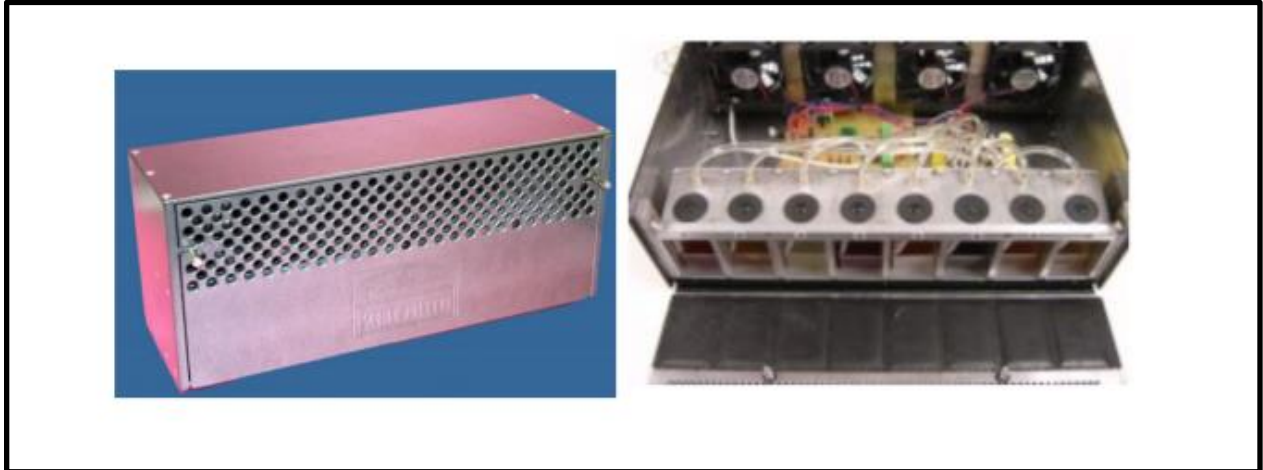
Figure 13: External casing of the Stimulus Delivery System on the left and inner components on the right. [35]
