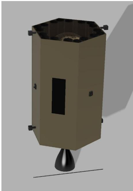
**Fig. 16 CAD model of Demeter, showing the deployment tubes along the inside edge and a one meter bar to show scale.**
