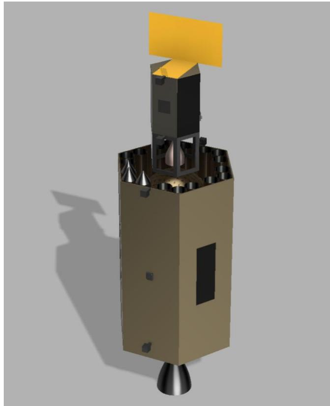
**Fig. 18 Satellite assembly with LEAVES probe clusters in three of the eighteen launch tubes.**
