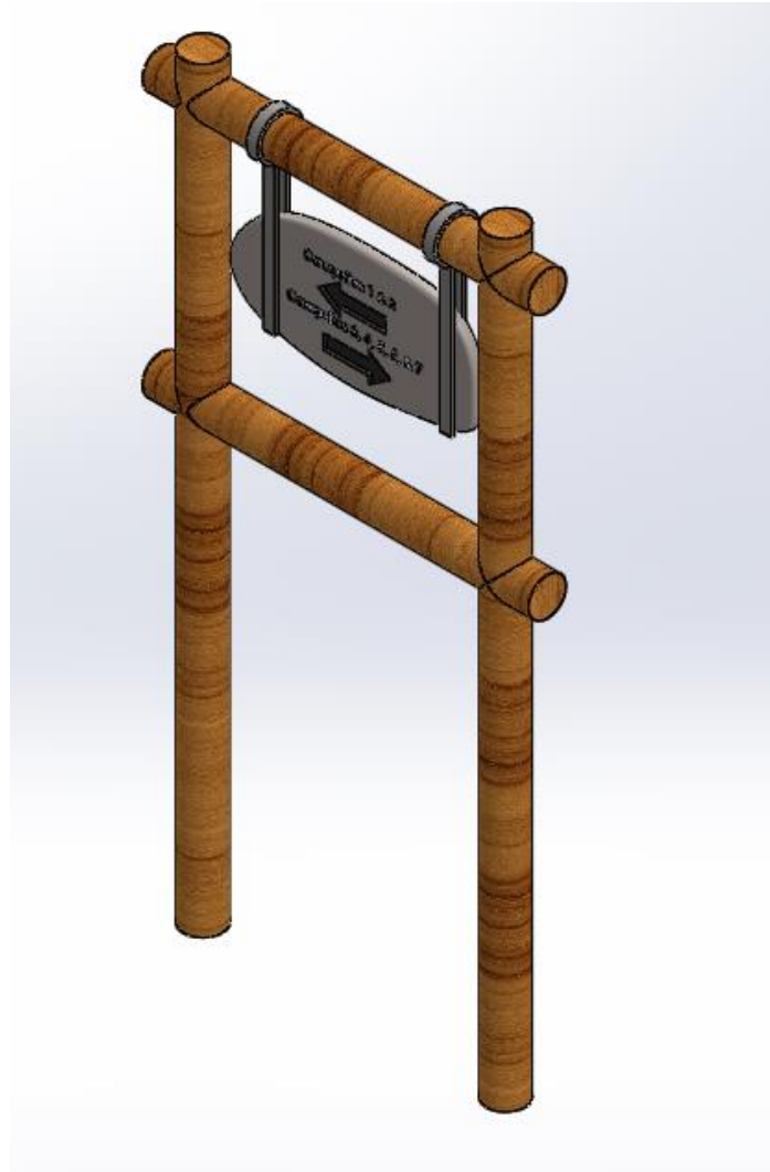
Figure 52: Elevated Wooden Sign Structure
