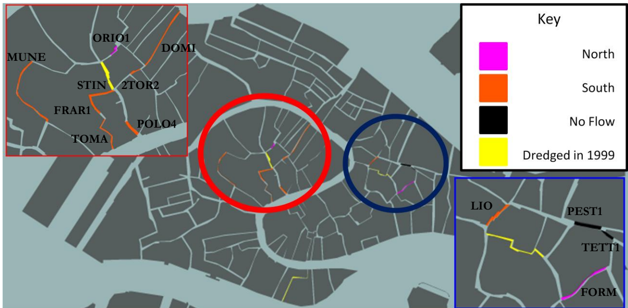
Figure 5.3: 1999 Outgoing Tide Flow Directions of Canal Segments Possibly Affected by Dredging in 1999
