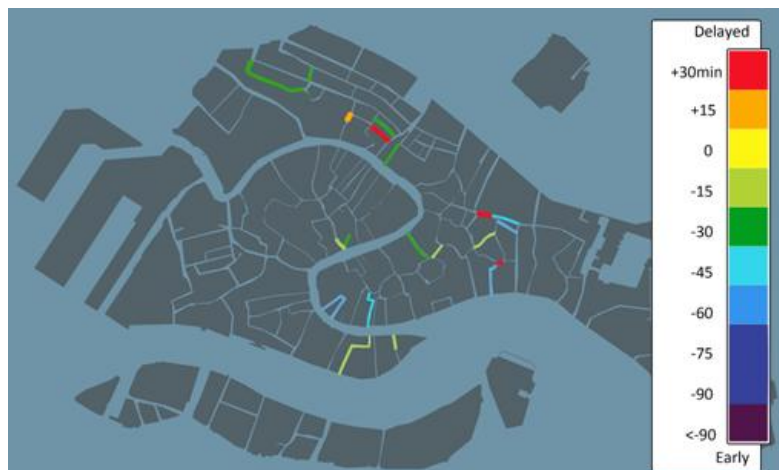
4.8 Map of low tide delay times with respect to the Punta della Salute low tide tim
