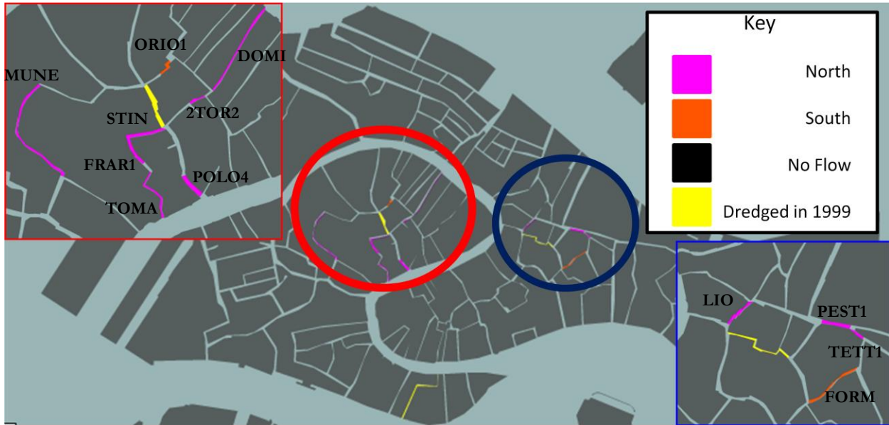
Figure 5.2: 2010 Incoming Tide Flow Directions of Canal Segments Possibly Affected by Dredging in 1999
