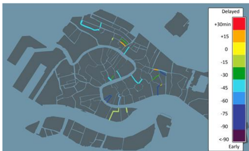
4.10 Map of low tide delay times with respect to the Misericordia low tide time
