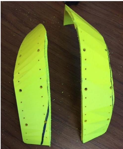
*Figure 39: First iteration of shoulder pads after initial modifications*
