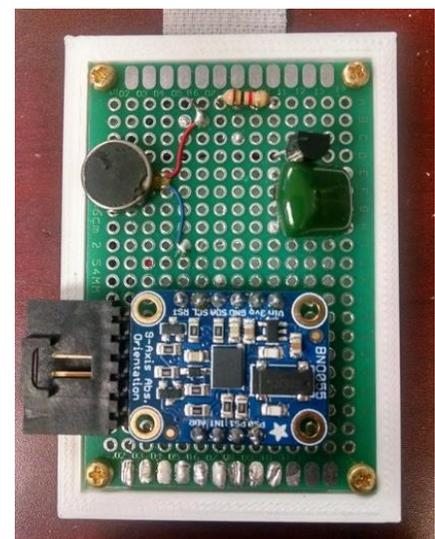
Figure 43: Protoboard containing IMU and vibration motor circuits
