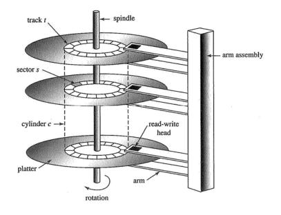
Figure 2.1 Moving-head disk mechanism [1, pg. 37]
