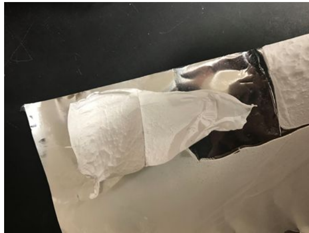
Figure 11: Electrospun product of alginate and PEO at concentration 20-20 mg/mL.
