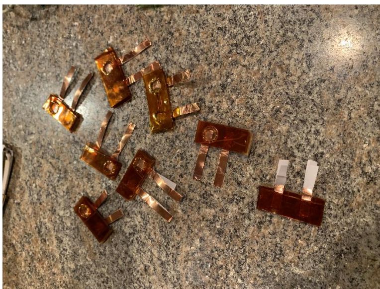
Figure 4A. We created many Gough cells at a time because of the leaking issues described above.
