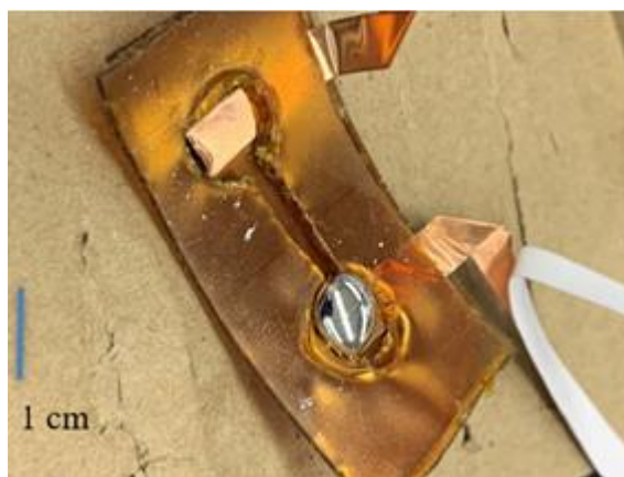
Figure 20. Galinstan droplet preparation inside of a Self-Actuation test module
