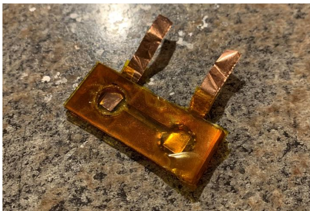
Figure 3A. The Gough cell once we finished punching holes into the layers and stacking each layer including the silicon layer.
