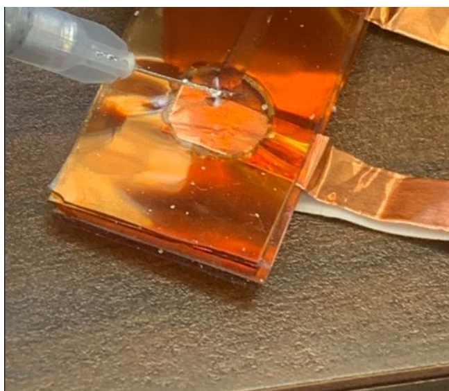
Figure 6A. Shows the process of placing the liquid Galinstan into the Gough cell through the silicon layer.
