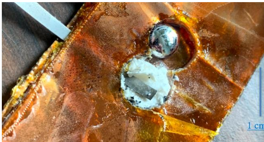
Figure 56. Shows the disintegrated separators due to long-term KOH exposure
