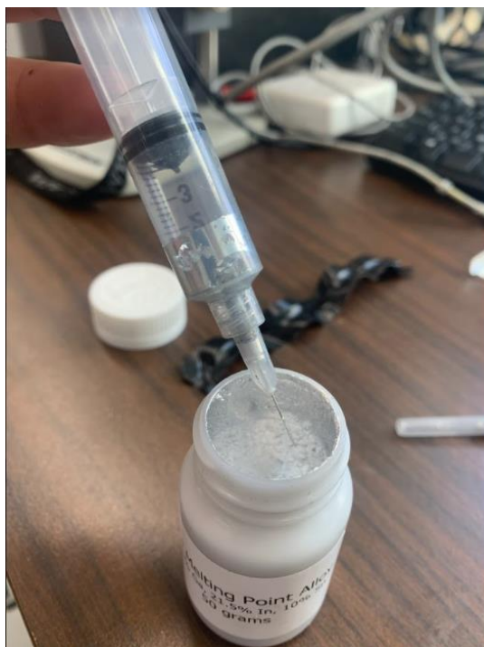
Figure 5A. Shows the process of collecting the Galinstan into the syringe so that it be moved into the Gough cell's anode.
