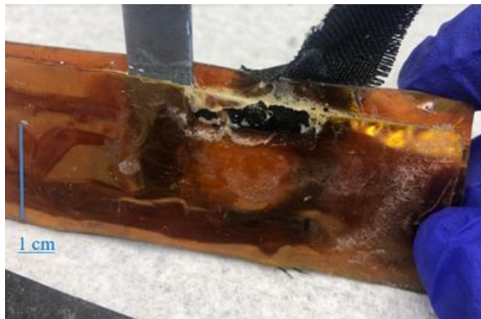
Figure 55. Evidence of KOH leakage through the polyimide layers
