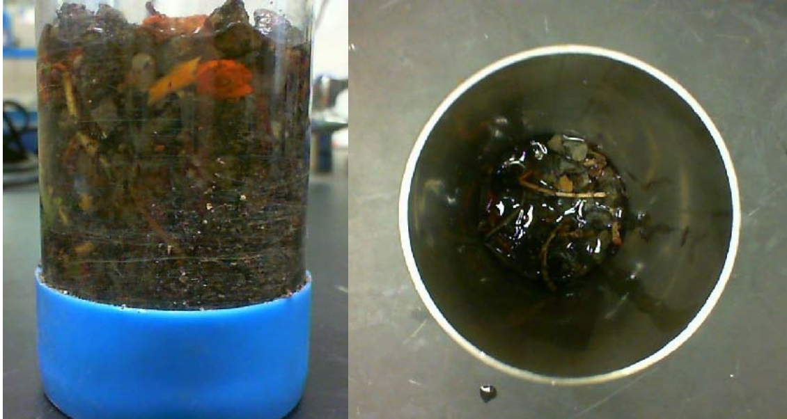
Figure 3.8: Saturated Green Roof Panel Cores
