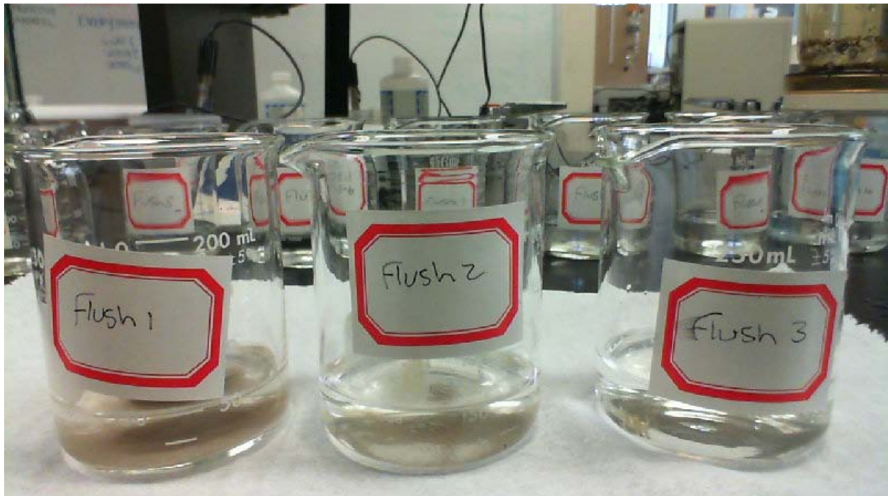
Figure 4.23: Runoff from Soil Flush Test
