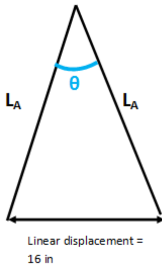
Figure 3: Schematic for determining torsion bar angular deflection \theta , based on linear displacement
