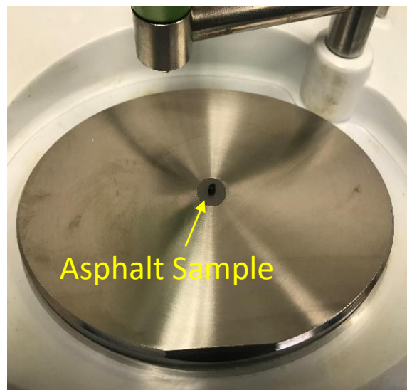
Figure 3.5: Extracted Asphalt Binder on ATR Crystal
