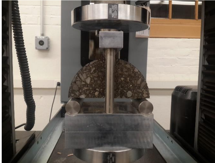
Figure 3.1: Semi-Circular Bending (SCB) Sample Test Setup
