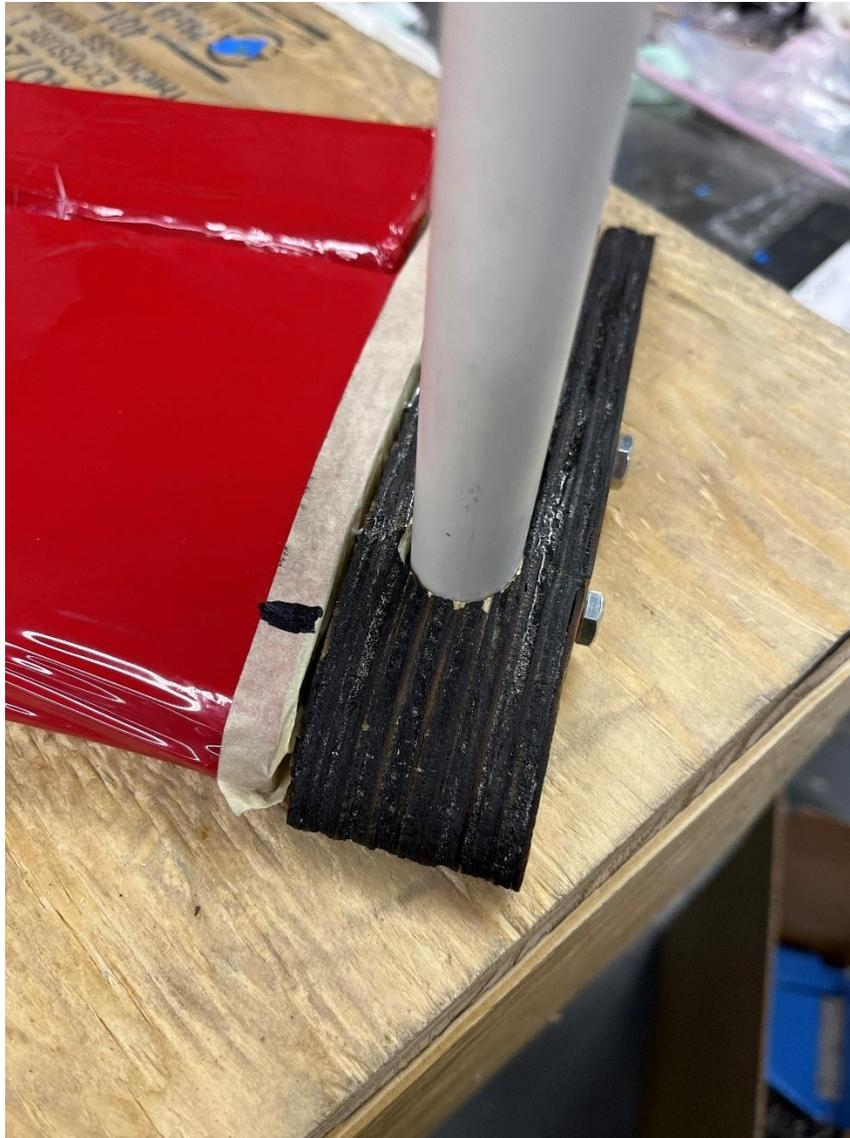
*Figure 83: Antenna Mount on Wing*
