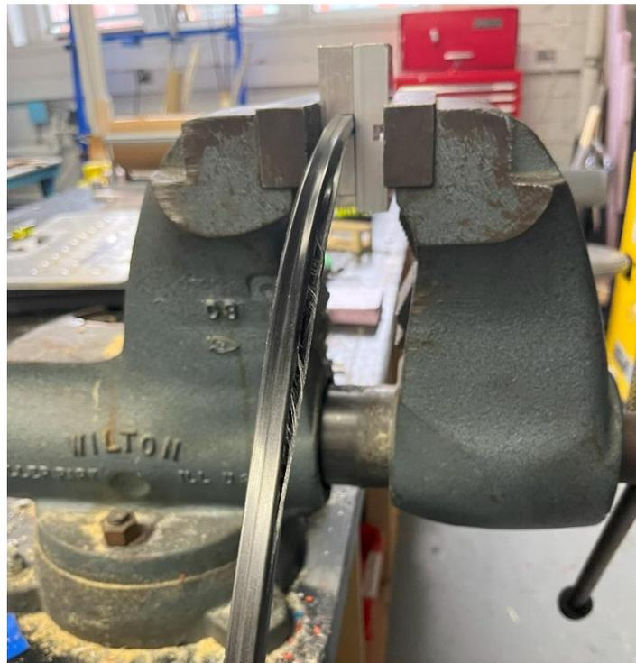
Figure 74: Square Carbon Fiber Rod Failure
