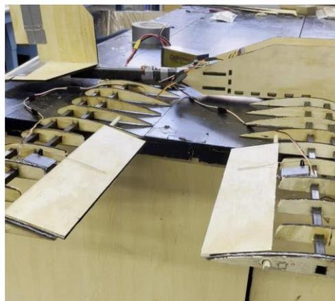
Figure 69: Example of a control surface functionality test
