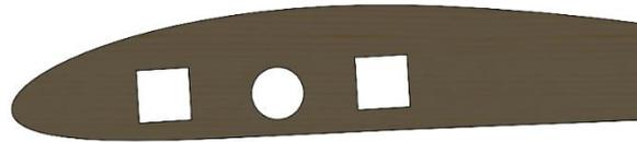
Figure 78: Cut Rib Side Profile
