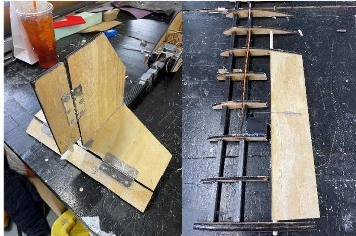
Figure 25: Photos of the initial wooden elevator, rudder, and aileron control surface setup
