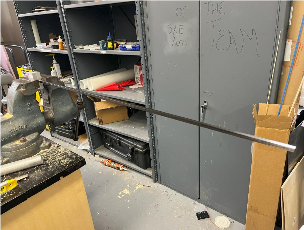
Figure 71: Cantilever Beam Test Setup
