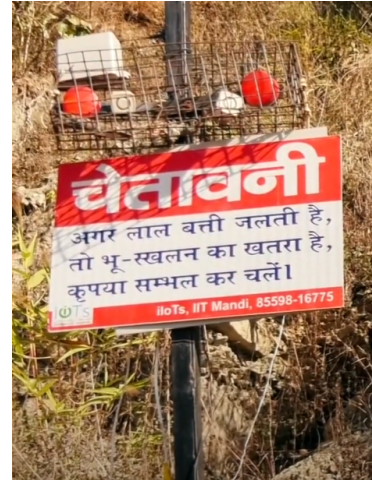
Figure 10: EWS Roadside Post
