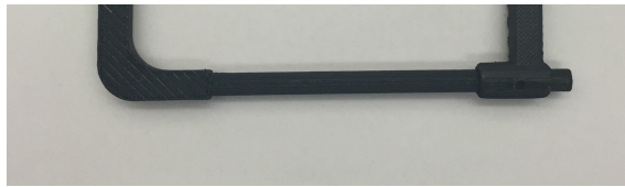
Figure 85: 3D printed square cuff design in extended position for retraction in larger patients
