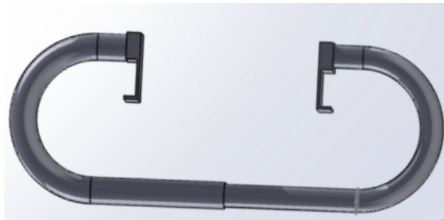
Figure 82: Cuff Retractor Iteration 2 in extended position for retraction in larger patients
