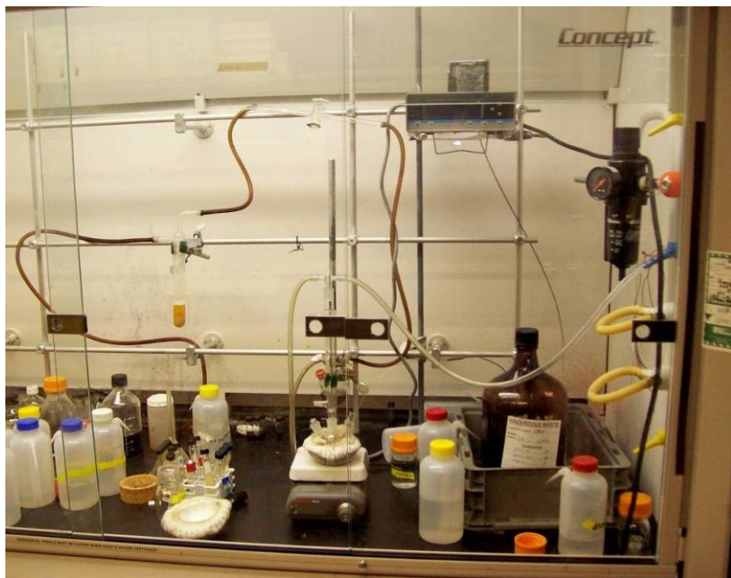
The pictures above show the pyrolysis reaction setup.
