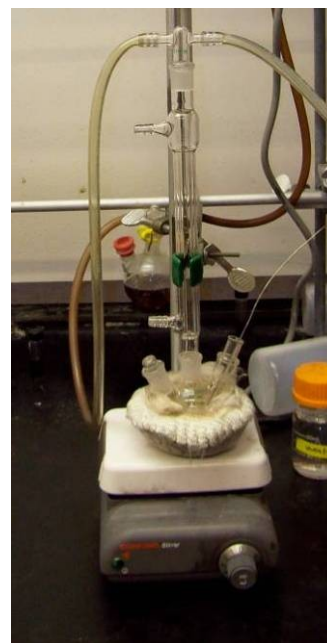
The pictures above show the pyrolysis reaction setup.
