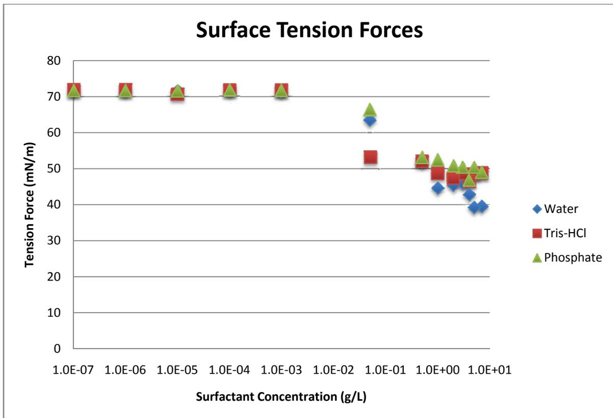
Figure 4.1 – Surface Tension Forces
