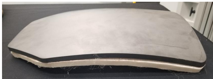
Figure 2 - A SAPI ceramic overlaying an UHMWPE composite before autoclaving
