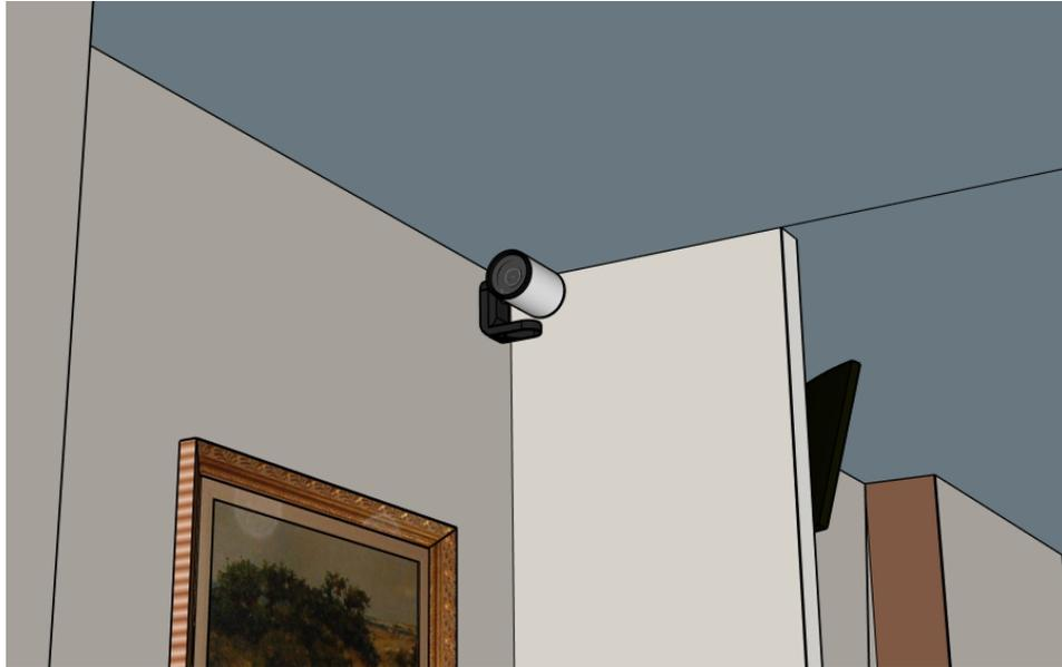
Figure 25. Recommended location of speaker-facing camera.
