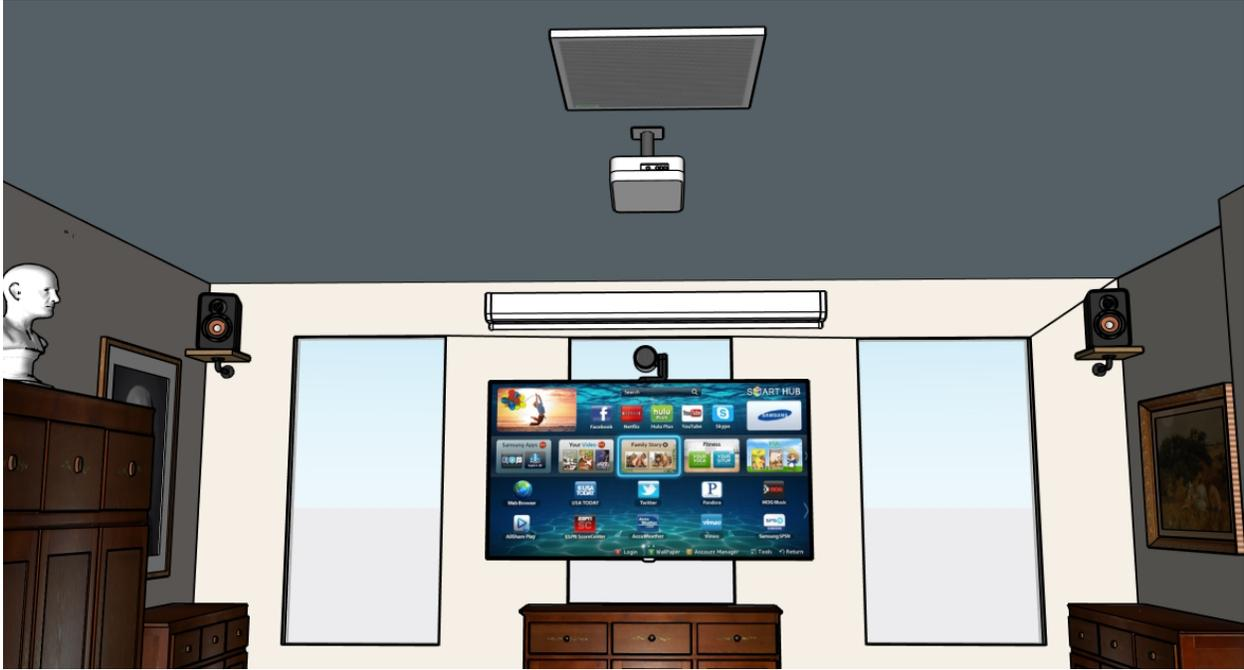
*Figure 23. Recommended Video Room front configuration.*
