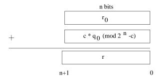
In general, this new expression for the residue class is still larger than  $2^n$ , and by implication larger than p. So we repeat this process once more, again rewriting the equations and replacing  $2^n$  by c:
