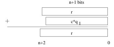
Finally we have an expression for the residue of  $a_ib_j$  that in general is less than  $2^{n+2}$ . To complete the reduction, we may need to subtract p from the intermediate result r one or more times. We simply test for this case and we have completed the reduction.
