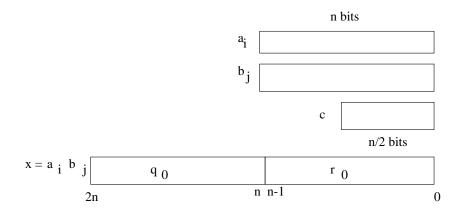
In this example, we begin with two subfield elements  $a_i$  and  $b_j$ , which are of size less than  $2^n$ , where  $2^n - 1$  is the maximum integer we can represent in a single machine register, and c is as in the above algorithm. We form the product  $x = a_i b_j$  which is of size less than  $2^{2n}$ , but in general larger than  $2^n$ , and by implication larger than p. So we use the above algorithm to perform a modular reduction.
