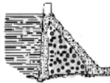
Figure 13 – Concrete capped, rock filled gravity dam. (Graham, 1997)
