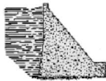
Figure 12 – Solid gravity dam. (Graham, 1997)
