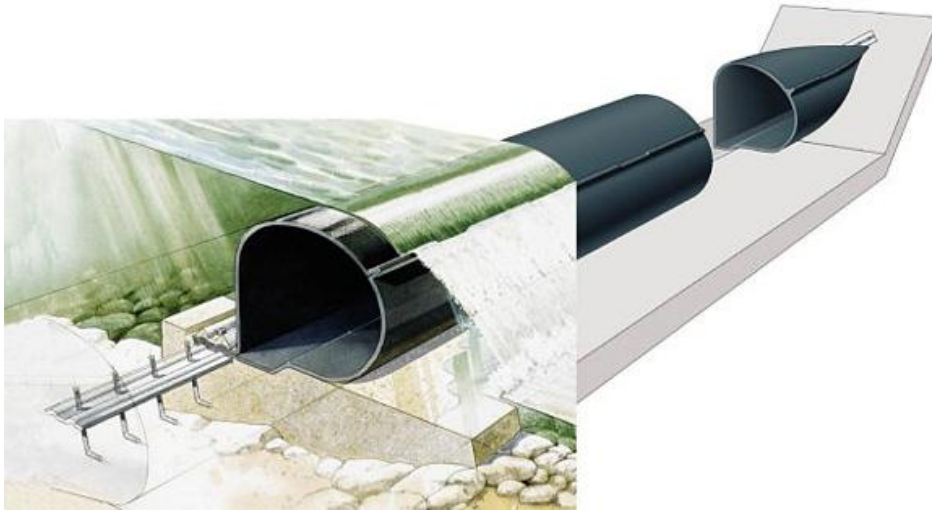
Figure 16 – Bridgestone-Firestone inflatable rubber dam.
