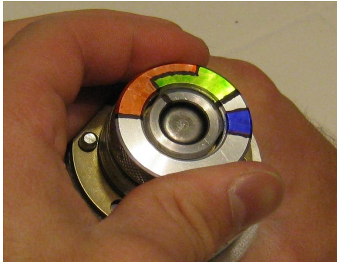
Figure 25: Photograph of clutch set to higher tension for lower half of leg ("green ankle" setting)
