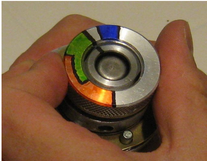
Figure 26: Photograph of clutch set to lower tension for upper half of leg ("green calf" setting)
