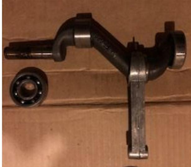
*Figure 25, Crankshaft Assembly*
