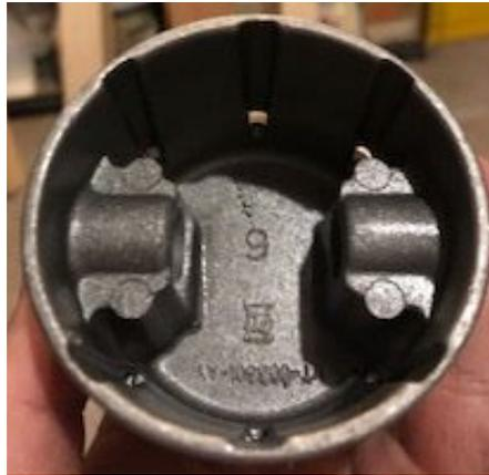
*Figure 22, Piston Bottom View*
