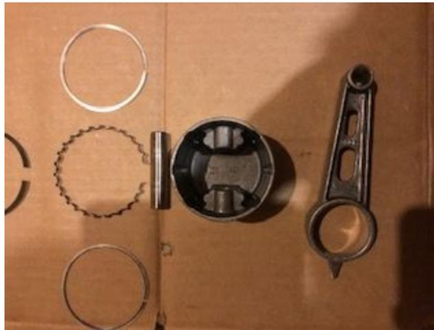
*Figure 21, Connecting Rods, Piston Heads, and Piston Rings*
