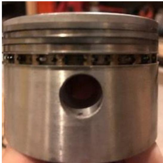
*Figure 24, Piston Ring Assembly*
