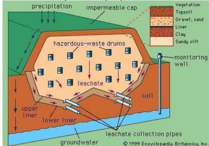
*Note.* This schematic depicts a leachate collection system. As can be seen, the hazardous waste is securely buried in a lined landfill that allows for the leachate from the waste to percolate down to the collection pipes in which it can then be removed and properly disposed of. This allows for a slow detoxification of LLW.
