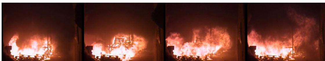
**Figure 1.** Still images from a video clip of pulsation (delta time  $\approx 1.4$  seconds); Short flames standing upright in the first clip. Then the flames lean towards the floor. As the longitudinal flow velocity reduces, the flames starts to stand up. The fire releases combustion products and its flame length becomes shorter as shown in the first clip.
