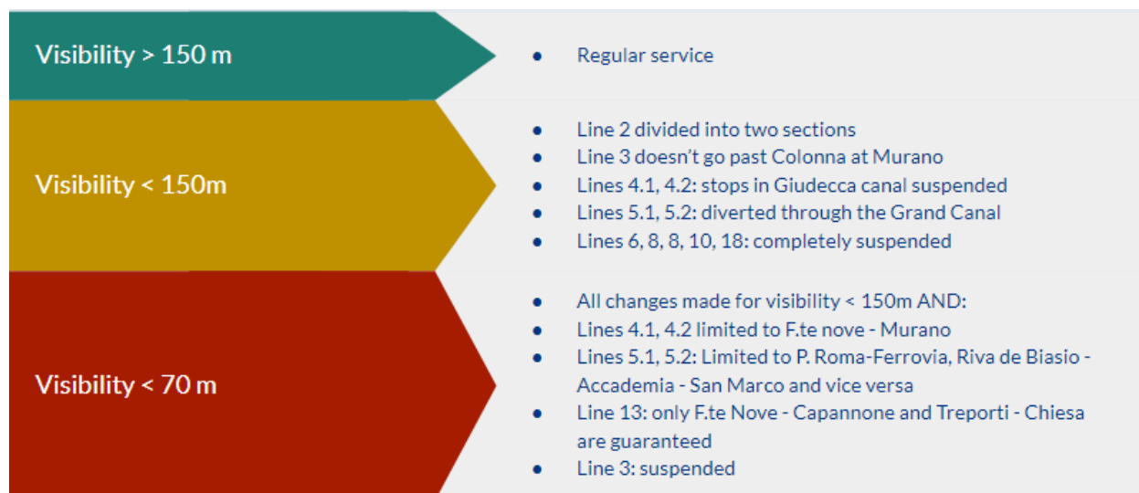
Figure 21: Changes to ACTV vaporetti operations based on visibility (Adapted from ACTV, n.d.)
