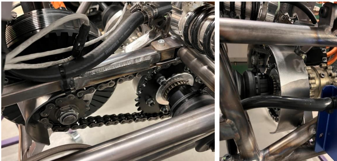
Figure 67: Scatter Shield Installed in Car
