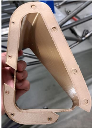
Figure 99: Duct Prototype Post Modification
