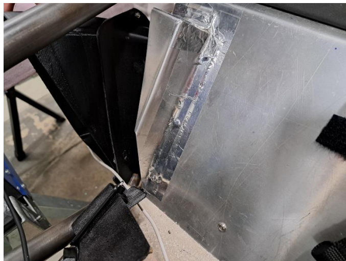
Figure 15: Accumulator Duct Cutout
