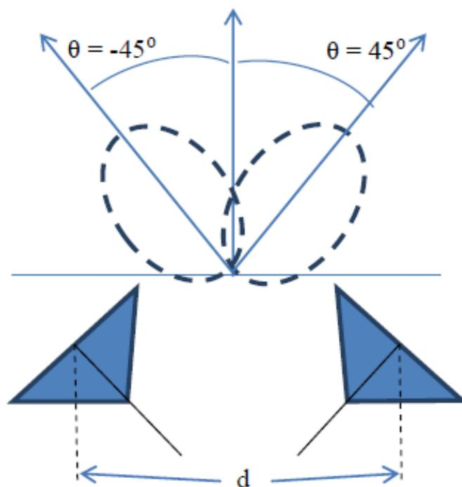
Figure 13: A two antenna amplitude comparison system. Each blue triangle represents a horn antenna. The antenna boresights are offset by  $90^\circ$ . Source: (Silva et al., 2011).
