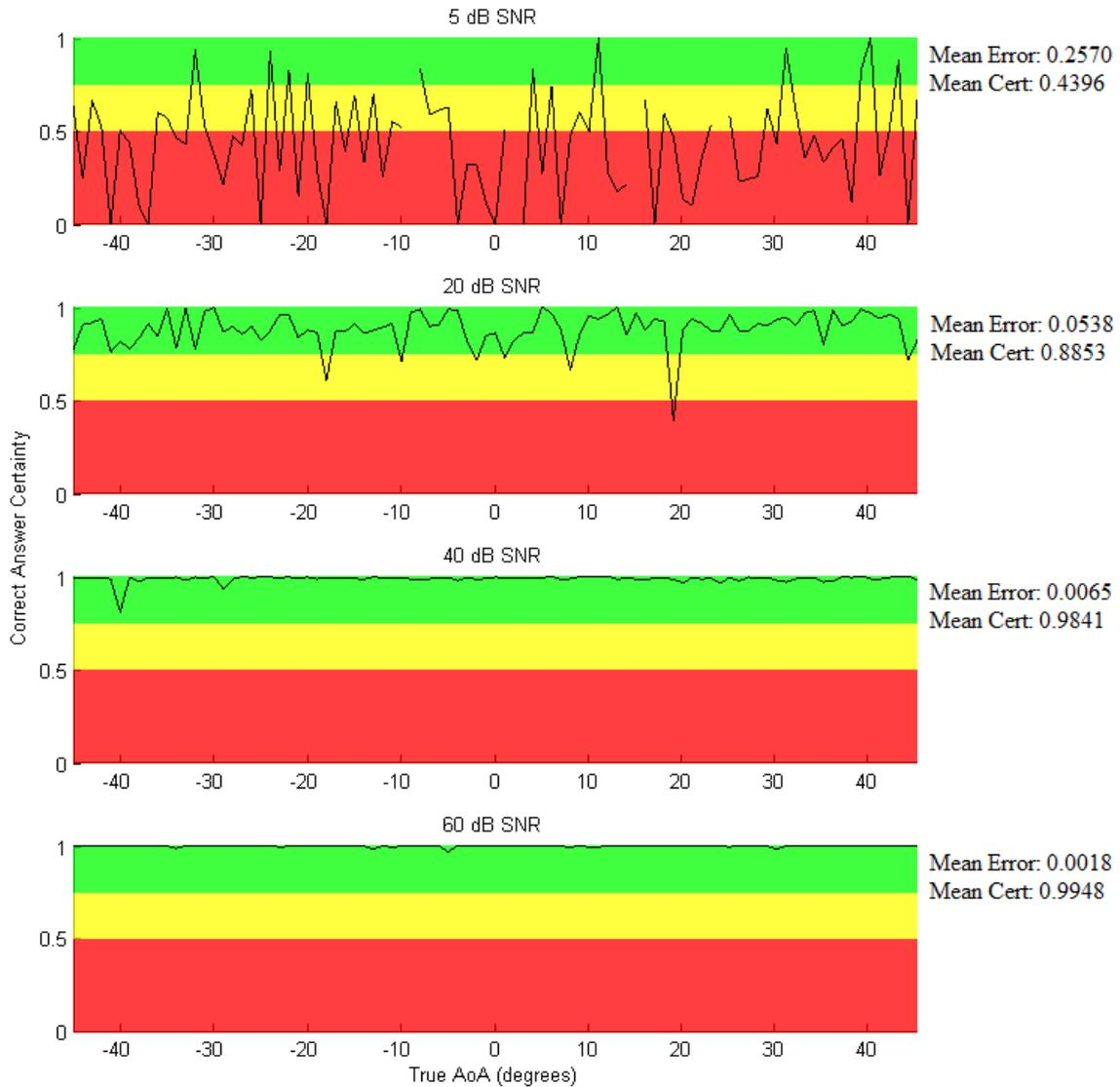
Figure 28: The graph of certainty in AoA calculations vs. true AoA for all angles between -45 and 45 degrees. Four SNRs were tested: 5 dB, 20 dB, 40 dB and 60 dB. When the SNR was set to 5 dB (Top), the signal was not detected in some cases, causing discontinuities in the graph. For SNRs within our 40 dB range, the system rarely dismissed signals as noise and rarely resolved the ambiguity incorrectly.
