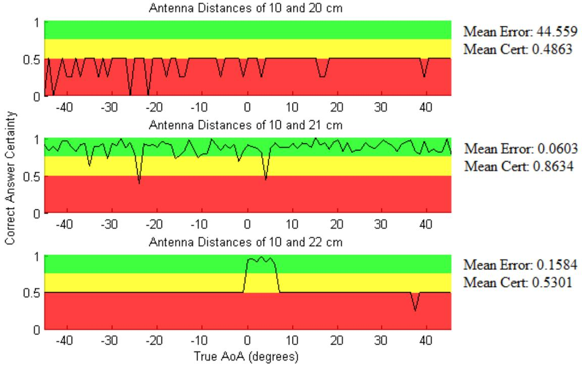
Figure 24: The graph of certainty of the correct AoA vs. the true AoA for all angles between  $-45$  and  $45$  degrees. Three different antenna (1-3) separations were tested, the calculated separation (21 cm) and the calculated separation  $\pm 1$  cm. The tests were run in worst case conditions. The average error and certainty are also reported for each of the antenna geometries. At 21 cm the mean error is minimized and the certainty is maximized as expected.
