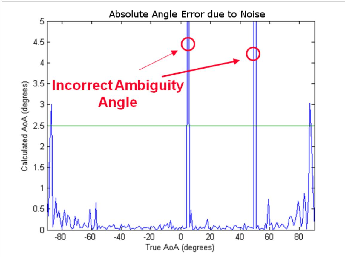
Figure 27: The graph of the primary calculated AoA versus the true AoA. The error is within the requirements of  $\pm 2.5^\circ$  (horizontal green line) for angles between  $-85^\circ$  and  $85^\circ$  except for the two cases where the ambiguity was resolved incorrectly (circled in red).
