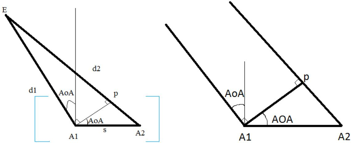
Figure 1: An interferometer system. (Left) An emitter distance  $d1$  and  $d2$  from two antennas separated by a distance  $s$ . Here,  $s$  is much less than  $d1$  and  $d2$ . (Right) The two antenna system close to the antennas where  $d1$  and  $d2$  are effectively parallel.
