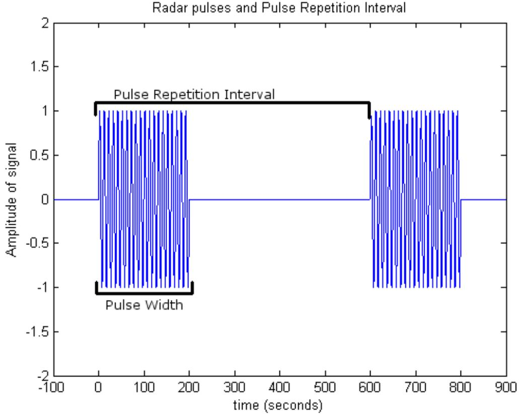
Figure 6: Two radar pulses with the same pulse width of 100 ms and a PRI of 400 ms. The first pulse arrives at  $t=0$  and the second pulse arrives at  $t=400$  ms.
