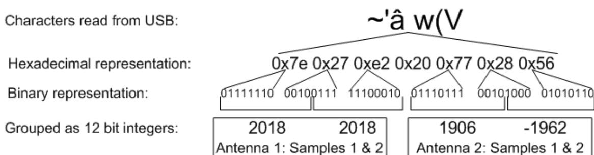
Figure 39: Sample data read in by the algorithm over the USB. The translation from USB read character to hexadecimal and binary is shown.
