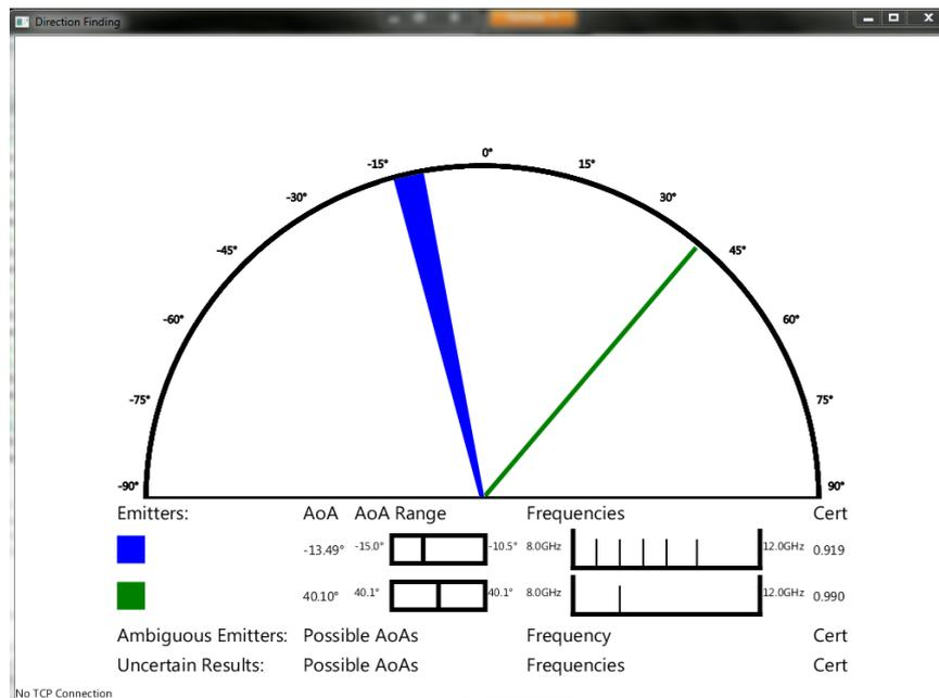
Figure 49: Display resulting from inputting mixed certainty results from  $-11^\circ$  to  $-15^\circ$ , a single certain result at  $40^\circ$ , and an uncertain result of either  $-45^\circ$  or  $80^\circ$ . The  $40^\circ$  result has been removed because more than 10 seconds have passed since receiving a signal from that location.
