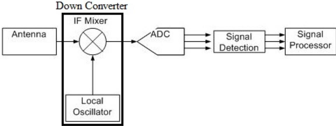
Figure 7: The setup of a superheterodyne receiver system. The antenna and local oscillator feed into the IF mixer. The mixer output is sampled by the ADC. If the signal detector finds a signal present, it is then passed off to the signal processor (Skolnik, 2001).
