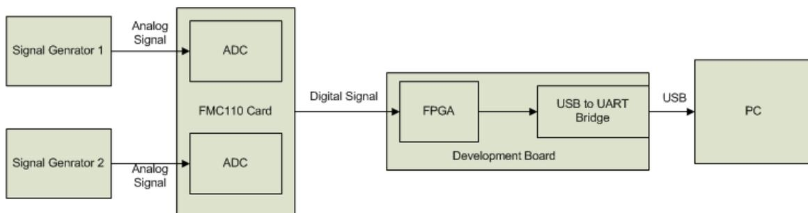
Figure 37: A block diagram showing the test setup of the two channel hardware implementation. The signal generators produce signals at IF. These signals are sampled by the ADCs and passed to a PC running the DF algorithm over a USB connection.
