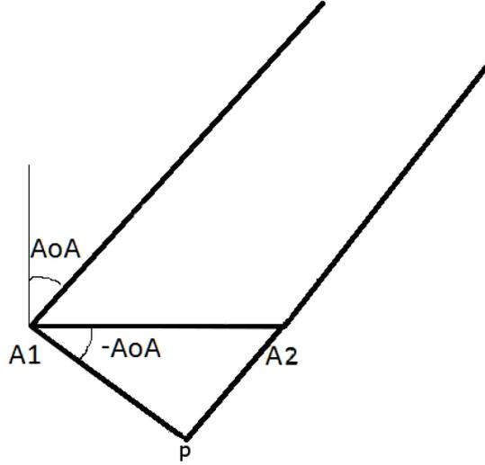
Figure 16: Figure 14 with the emitter moved to the right side of the interferometer. The line segment  $\overline{EA2}$  is artificially extended to point p so that antenna 1 can still be used as a reference. Emitters to the right of the interferometer result in negative total phase difference and negative AoAs.
