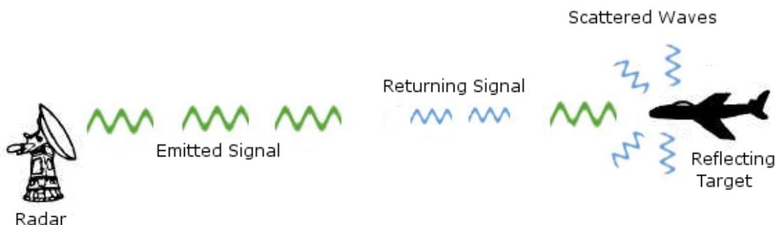
Figure 5: A basic depiction of a radar system detecting an aircraft. The emitted signal (large green waves) hits the aircraft and scatters in every direction (smaller blue waves). Some of the scattered signal returns to the emitter.
