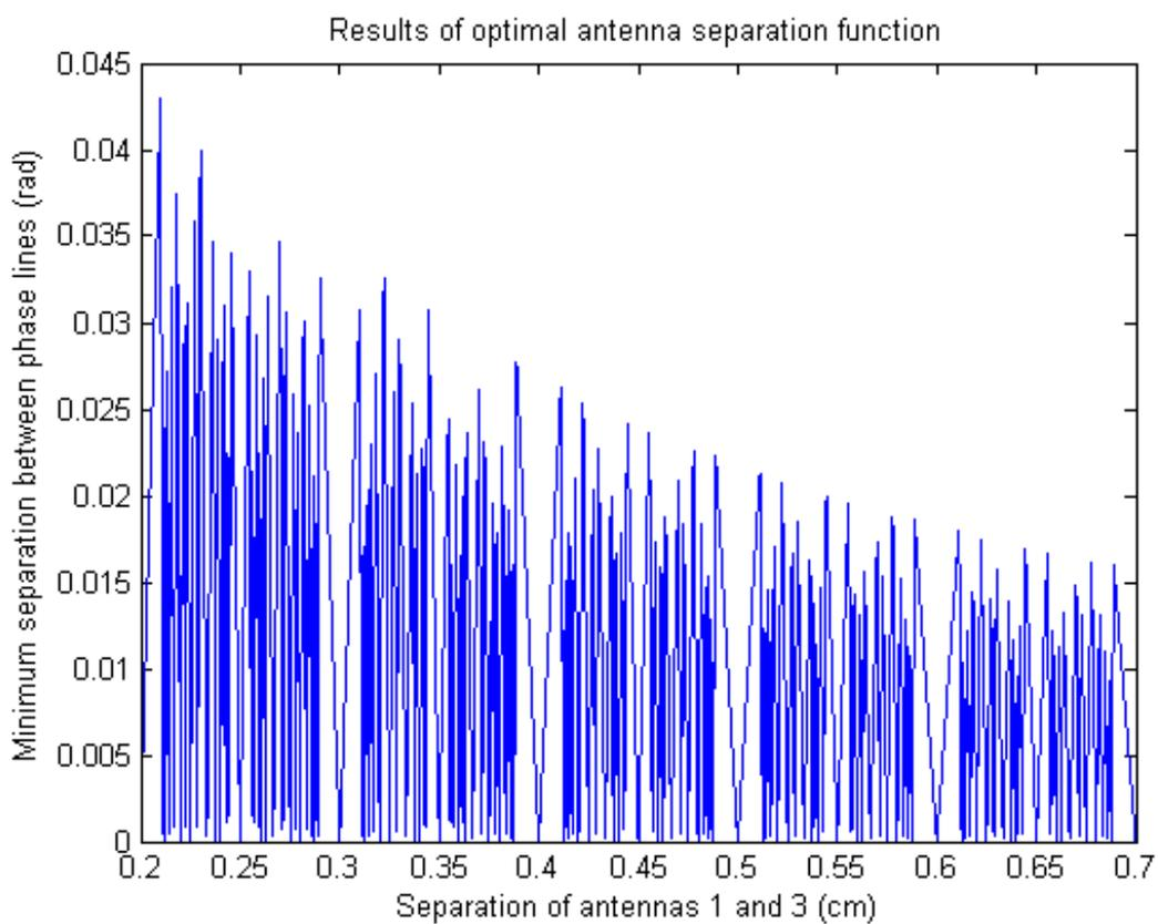
Figure 22: Plot of separation between antennas 1 and 3 versus the minimum separation between phase lines. This plot shows the result of the optimal antenna spacing function. The results shown are for  $s_{12} = 10$  cm and a maximum frequency of 12 GHz. The highest peak corresponds to the value for  $s_{13}$  that maximizes the phase line spacing.
