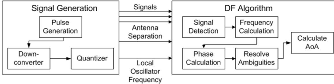
Figure 20: A block diagram showing the structure and components of the MATLAB model. The signal generator generates signals and replicates the processing performed by hardware as signals are received. The DF algorithm analyzes the three signals produced by the generator and determines the AoA
