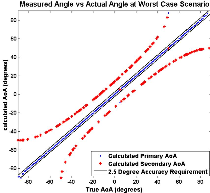
Figure 4: The primary (blue diamonds) and secondary (red stars) reported AoAs plotted against the known true angle with  $1^\circ$  steps in worst case conditions. In every case except for two, where the true AoAs were  $5^\circ$  and  $50^\circ$ , the most likely of the two angles reported by the system was correct. The black lines show the boundaries of the required  $\pm 2.5^\circ$  accuracy.
