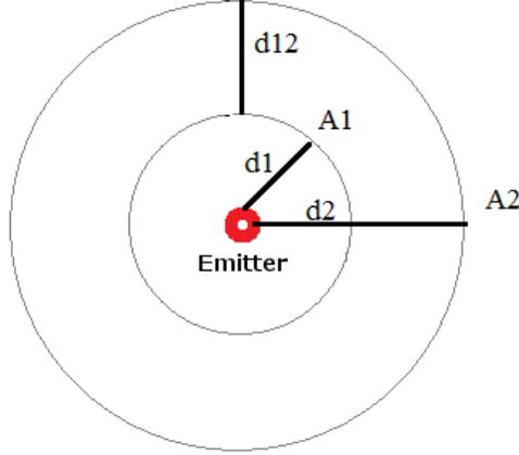
Figure 12: An example of a TDOA system. Antennas  $A_1$  and  $A_2$  are distance  $d_1$  and  $d_2$  away from the emitter. Each antenna sits on one of two concentric circles centered on the emitter. The radial distance between these circles is given by  $d_{12}$ .
