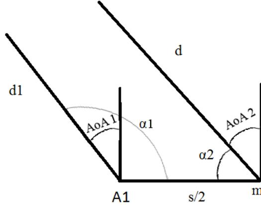
Figure 17: This figure shows the antenna 1, A1, and the midpoint between the two antennas, m. The distance from the emitter, not shown, to the first antenna is  $d_1$  and the distance from the emitter to the midpoint is  $d$ . The separation between A1 and m is  $s/2$  and the angle of arrival for each point is shown (AoA1 and AoA2 respectively). The angles of the triangle formed by the emitter, m, and A2 are  $\alpha_1$  and  $\alpha_2$ .
