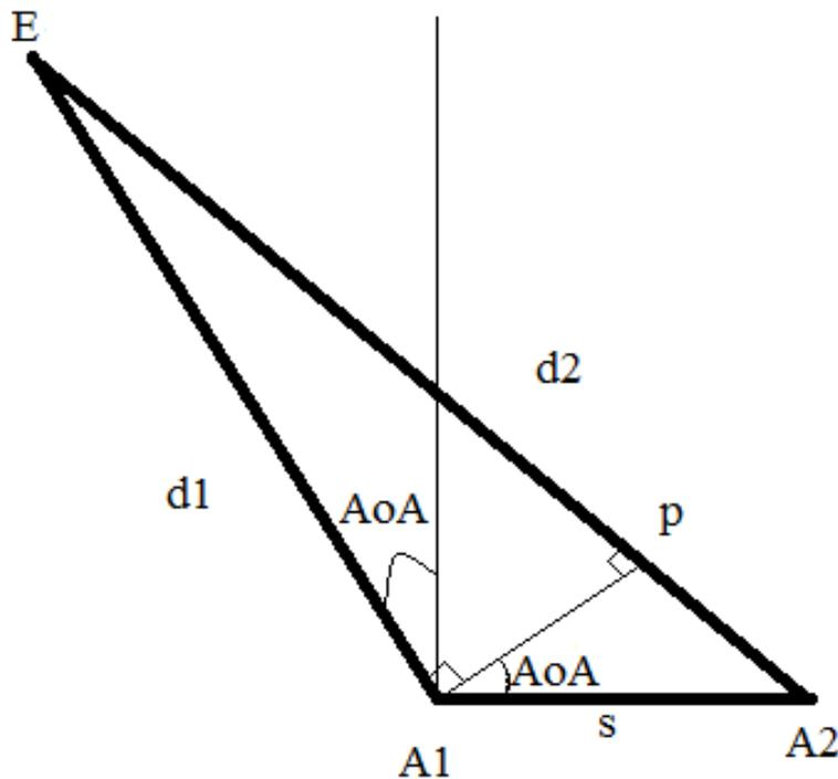
Figure 14: A phase interferometry system. An emitter distance  $d_1$  and  $d_2$  from two antennas separated by a distance  $s$ . Point p is placed on the line segment  $\overline{EA_2}$  such that  $d_1$  is equal in length to the line segment  $\overline{Ep}$ . Here  $s$  is much less than  $d_1$  and  $d_2$ .
