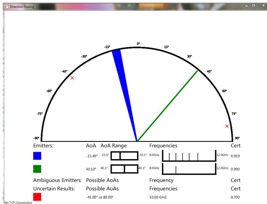
Figure 48: Display resulting from inputting mixed certainty results from  $-11^\circ$  to  $-15^\circ$ , a single certain result at  $40^\circ$ , and an uncertain result of either  $-45^\circ$  or  $80^\circ$ .
