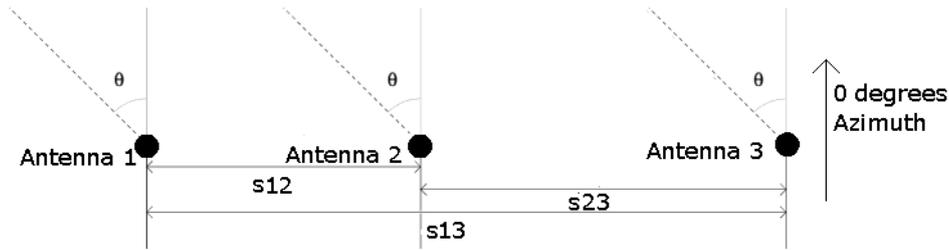
Figure 2: Setup of a three antenna interferometer.
