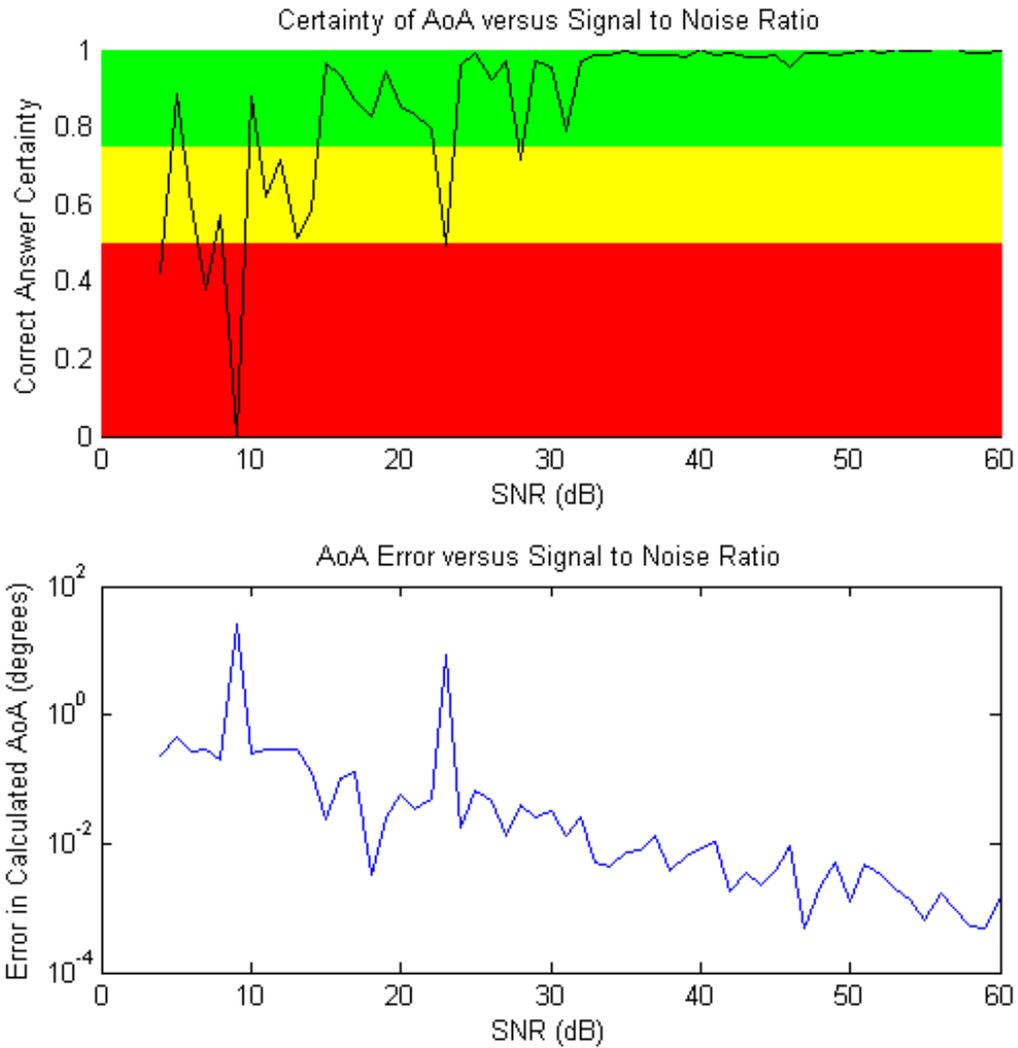
Figure 29: The graphs of certainty and error in AoA calculations vs. the SNR for an AoA of  $45^\circ$  between 5 dB and 60 dB with an SNR step size of 1 dB. The error axis is logarithmic. The certainty rises with SNR and the error decreases in an exponential manner.
