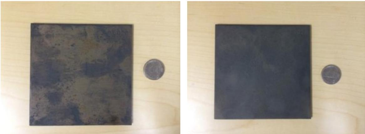
*Figure 118. Exposed Unaluminized RA602CA and aluminized RA602CA*
