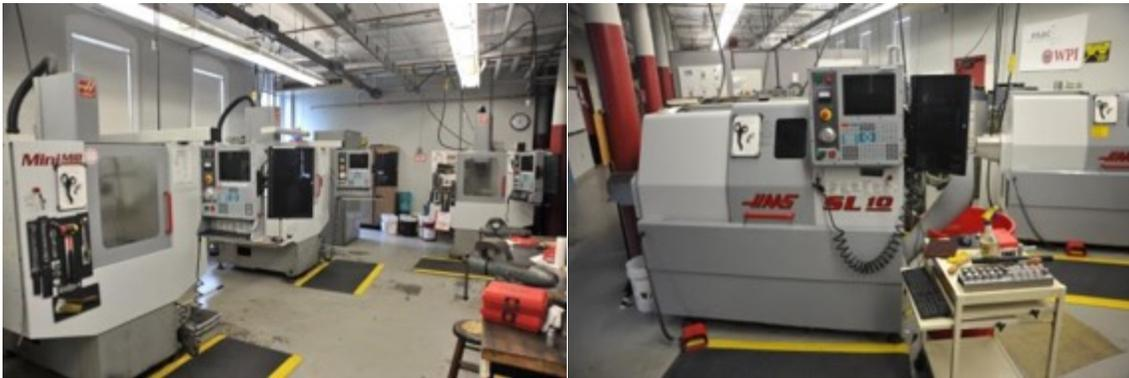
*Figure 16 HASS Mini Mill for surface finish (left) HASS Lathe for cutting (right)*
