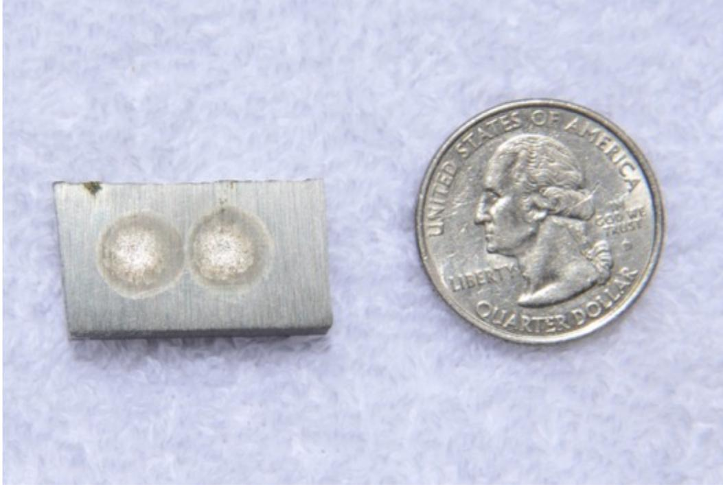
Figure 38: Photo of a piece of racking pole sample after twice OES measurements
