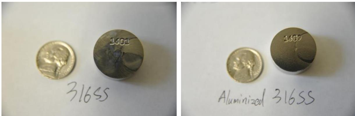
*Figure 14. Stainless Steel 316 (left) Aluminized Stainless Steel 316 (right)*
