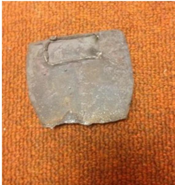
Figure 21. Photographs of Failed fan blade
