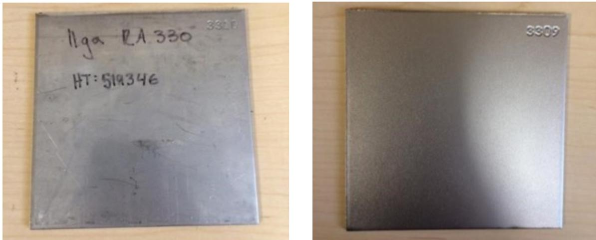
*Figure 10. Unaluminized (left) and aluminized (right) RA 330 samples*
