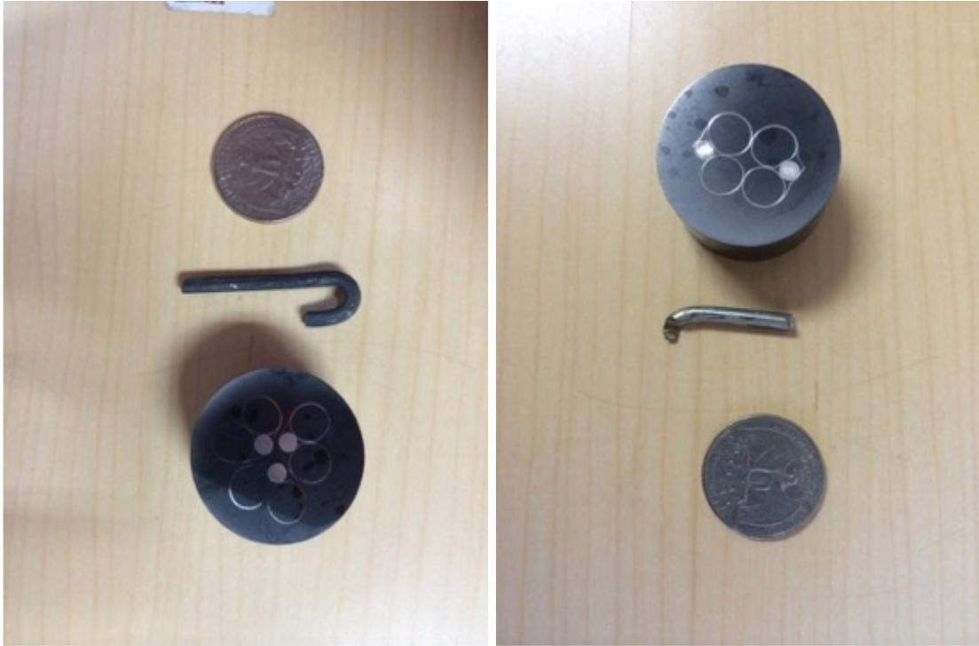
*Figure 53. Spirals cut from new (left) and failed (right) mesh belts and mounted in cross section*
