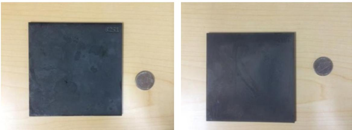
*Figure 119. Exposed Unaluminized and aluminized INCONEL alloy 625*
