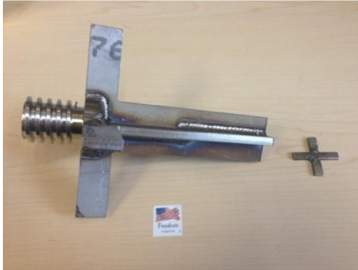
Figure 59. Sample cut from the racking pole by wire EDM
