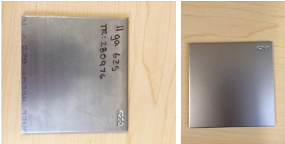
Figure 11. Unaluminized (left) and aluminized (right) INCONEL alloy 625 samples
