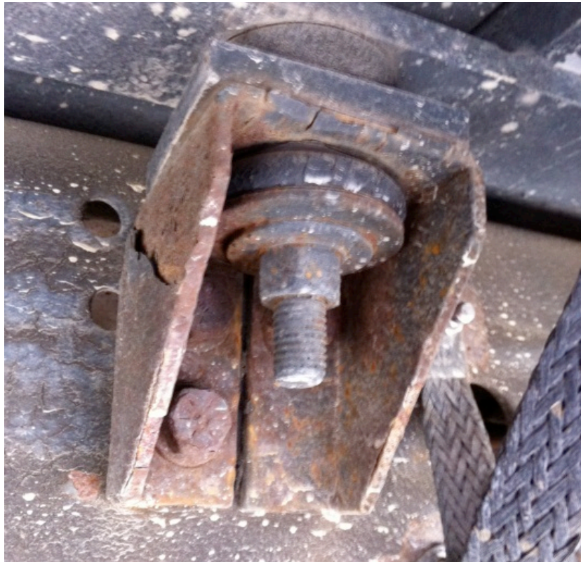
Figure 36- An example of mounting mechanism arrangement of an ambulance sub-frame to a vehicle chassis
