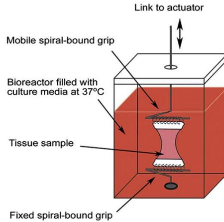
FIGURE 6: CUSTOM BUILT CELL ADHESION ANCHORING SYSTEM DEVELOPED FOR BIOREACTOR
