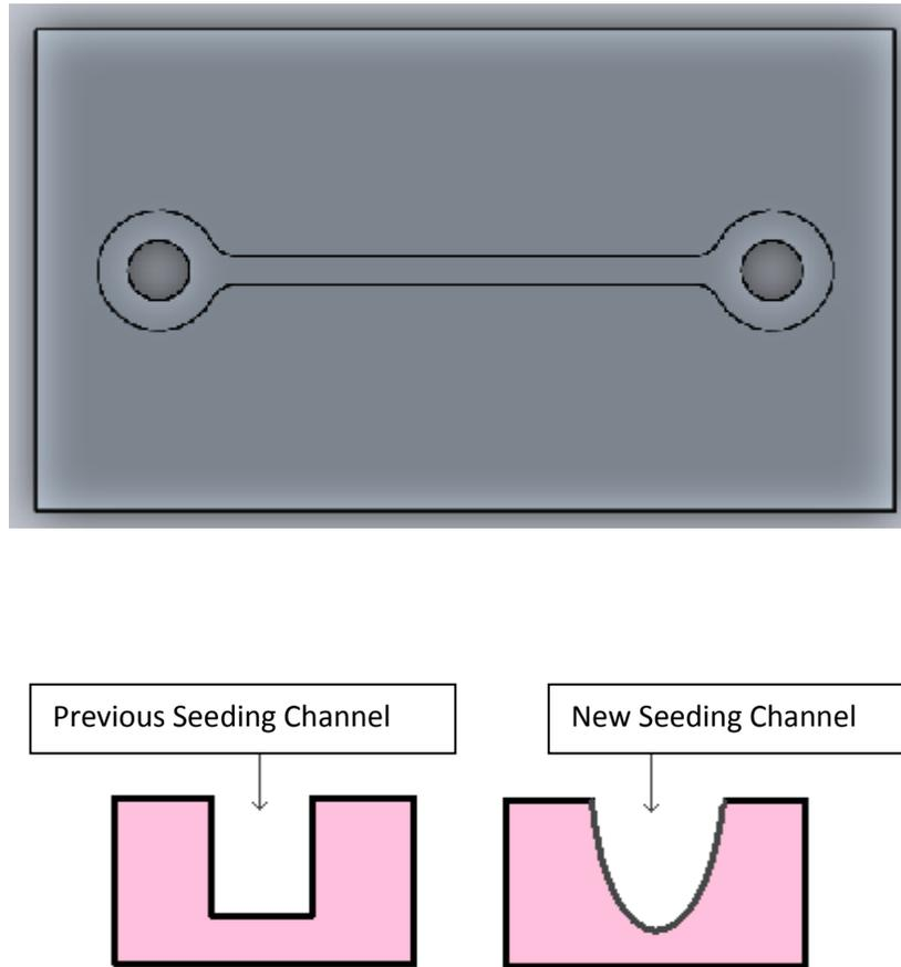
**FIGURE 10: EXAMPLE OF PREVIOUS AND NEW SEEDING CHANNELS**
