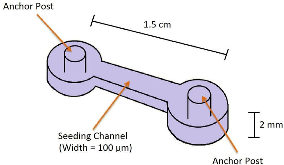
FIGURE 7: "DOG-BONE" MOLD ANCHORING SYSTEM
