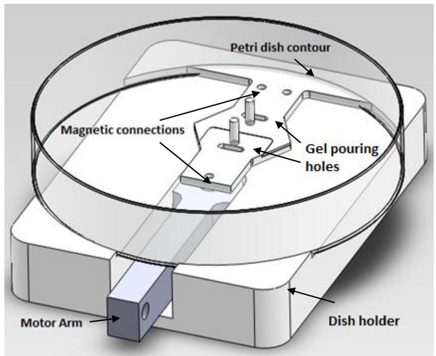
FIGURE 14: FINAL DESIGN, MAGNETIC CONNECTION TO MOTOR ARM AND PETRI DISH
