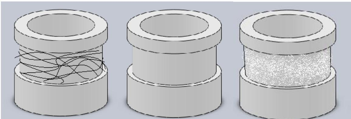
FIGURE 16 FROM LEFT TO RIGHT: ELECTROSPUN PE/PU, BARE PP, AND HYDROXYAPATITE COATED TISSUE RINGS
