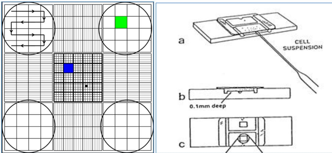
FIGURE 17: IMAGE OF HEMOCYTOMETER DEVICE (LEFT) AND 9X9 GRID (RIGHT)
