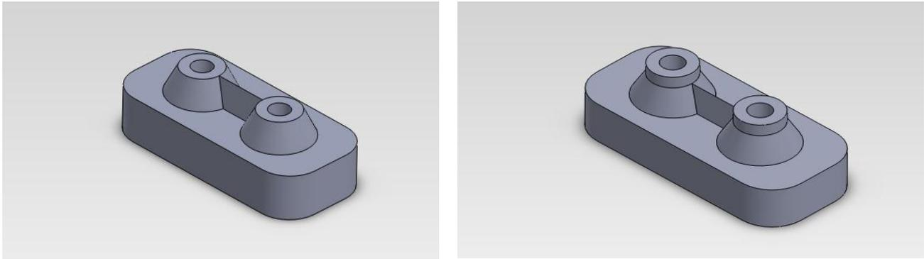
**FIGURE 23: AGAROSE MOLD NEGATIVE WITHOUT (LEFT) AND WITH (RIGHT) TISSUE RINGS**
