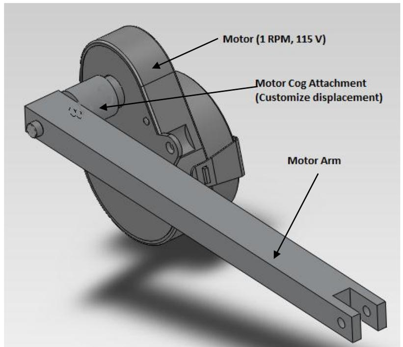
FIGURE 12: MOTOR AND CAM SYSTEM
