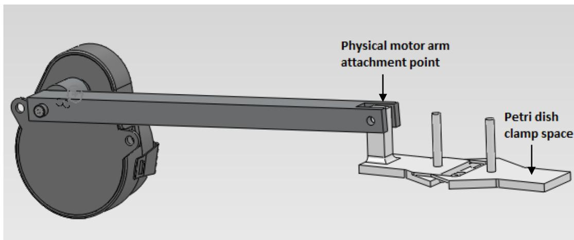
FIGURE 13: PRELIMINARY DESIGN, PHYSICAL ATTACHMENT AND PETRI DISH CLAMP
