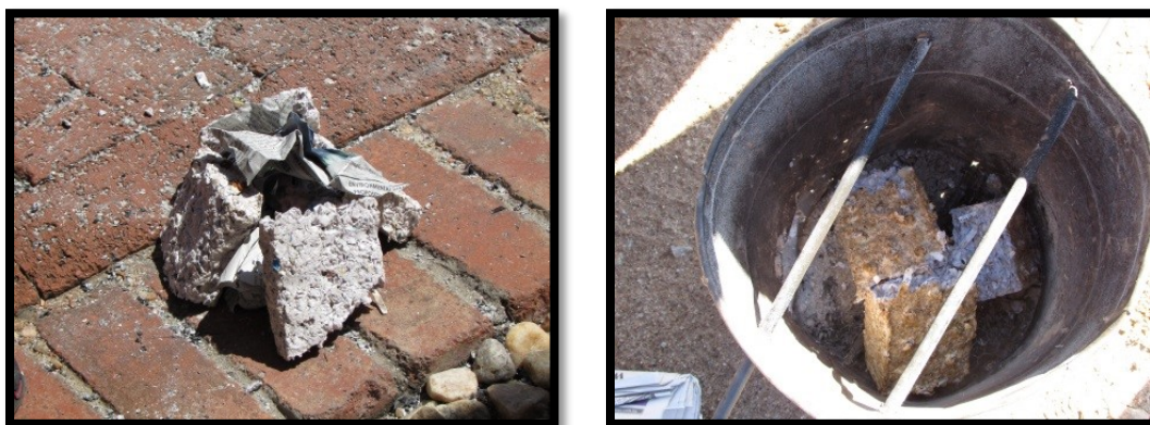
Figure 12: Testing setup for open air and stove based burn tests
