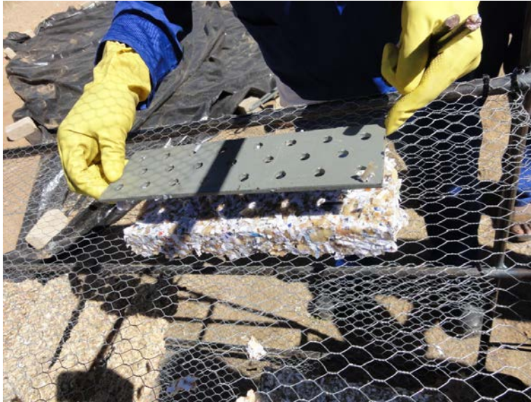
Figure 60: Removing top plate from newly molded block
