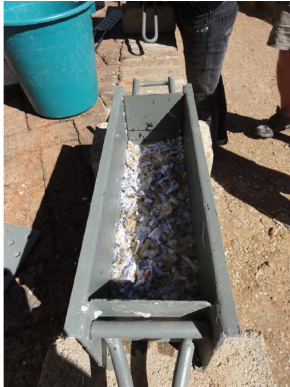
Figure 50: Mold filled to first line with mixture
