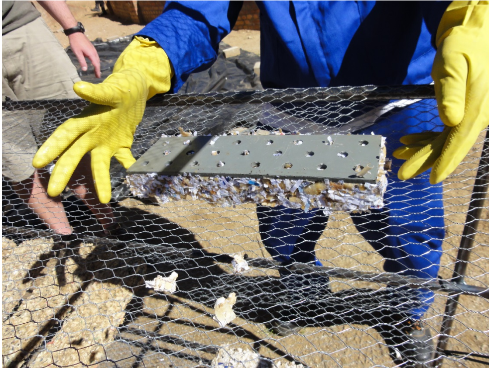
Figure 58: Pushing rods out of the block
