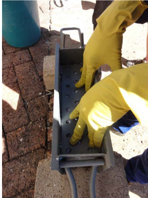
Figure 54: Compressing the mixture in the press
