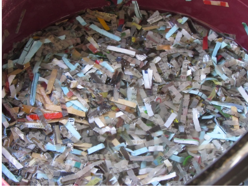
Figure 47: Mixture after soaking for 3-5 days and becoming pulpy
