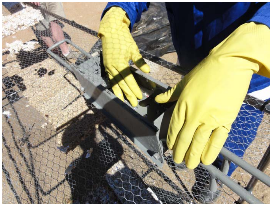
Figure 57: Pushing block out of mold
