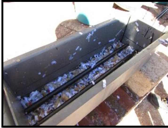
Figure 26: Metal rods being inserted during the molding process
