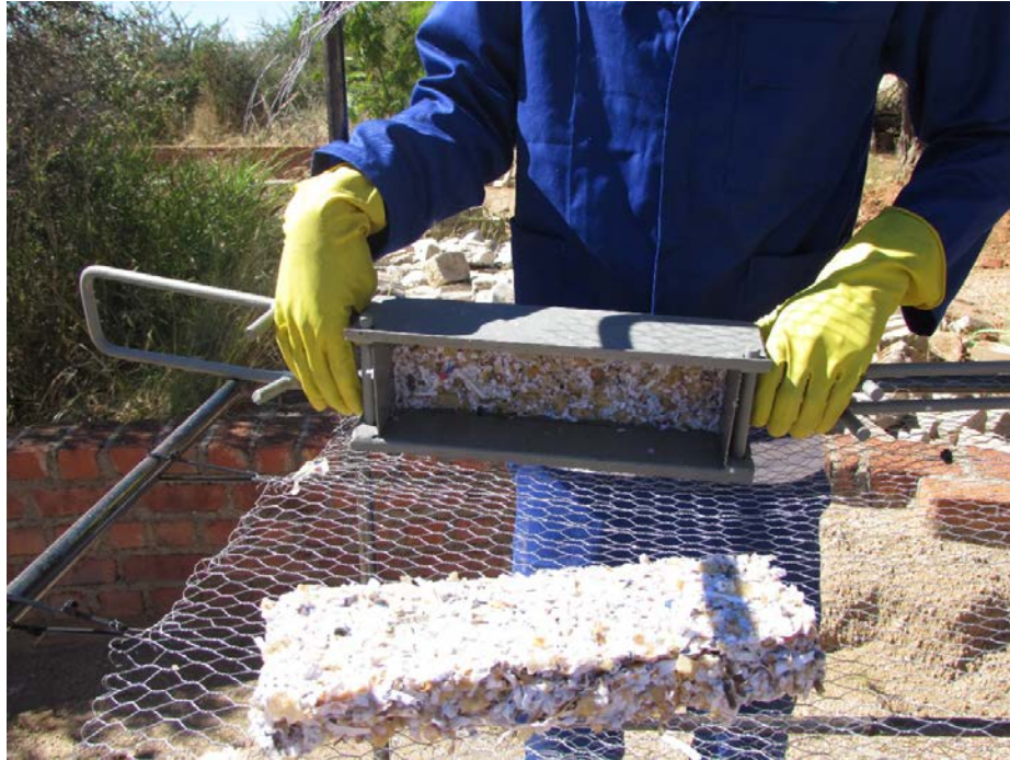
Figure 56: Block being turned over to remove from mold
