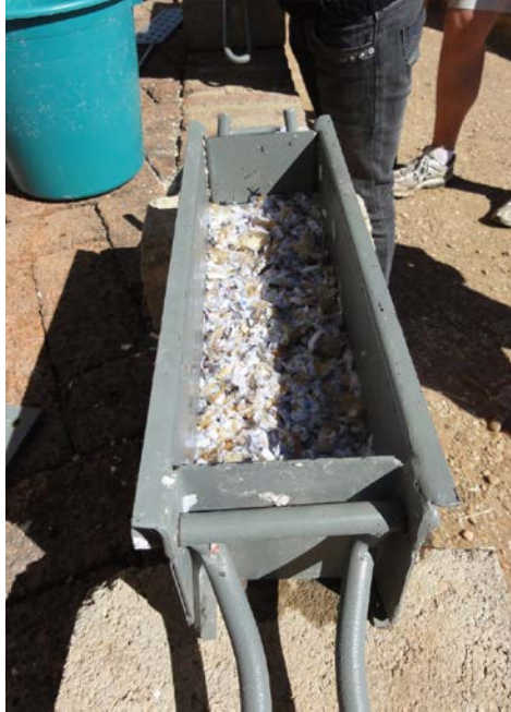
Figure 52: Mold filled with mixture to second line
