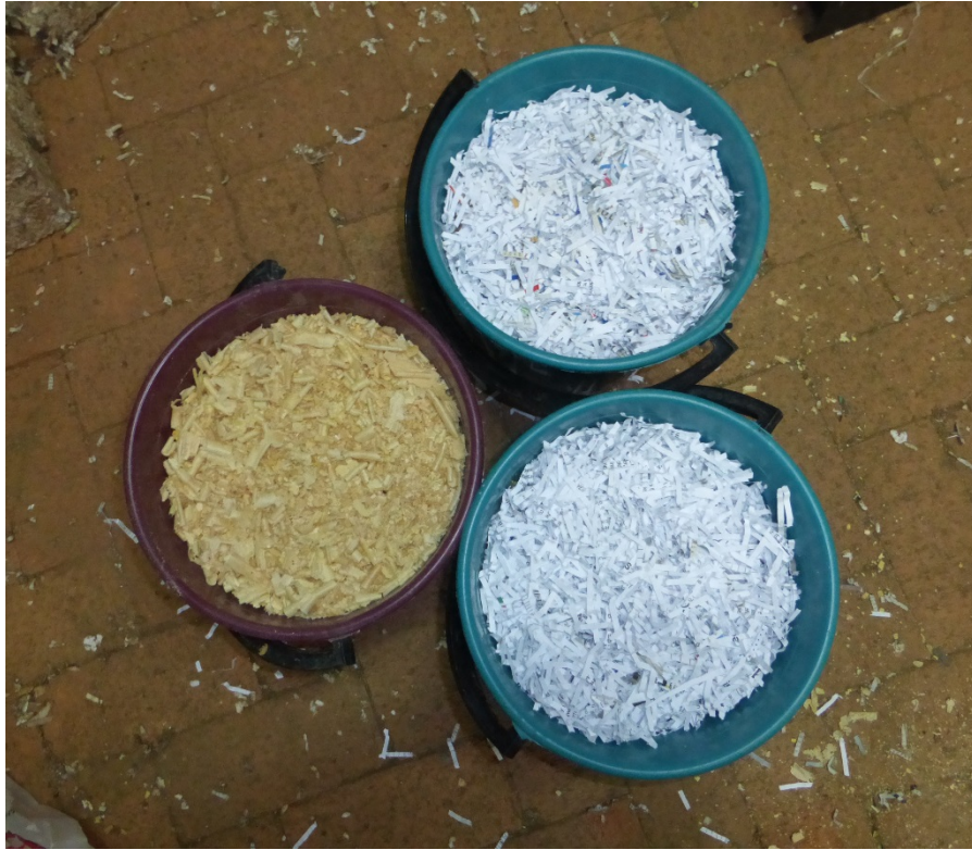
Figure 46: Buckets of Shredded Paper and Wood Shavings/Sawdust in 2:1 Ratio
