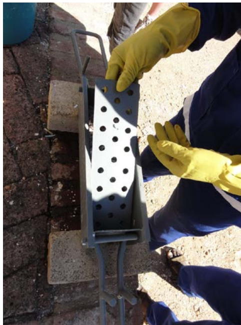
Figure 53: Placing the top plate on the mixture
