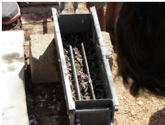
Figure 51: Rods placed on top of mixture
